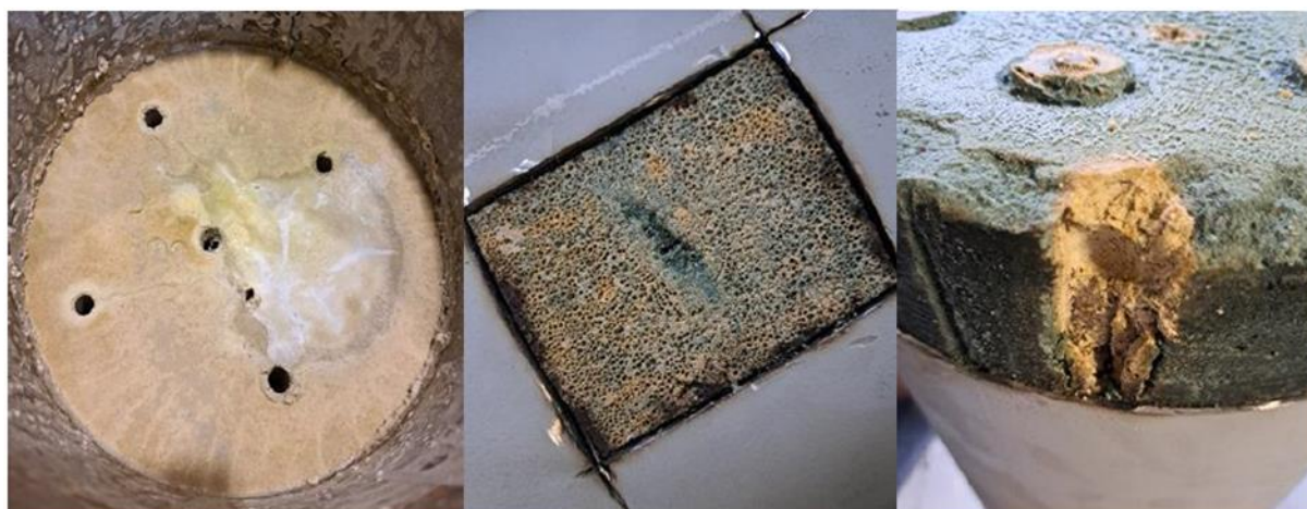
Figure 14: BFS-based GP with 10 wt.% oil loading inside 50 L drum [19]
