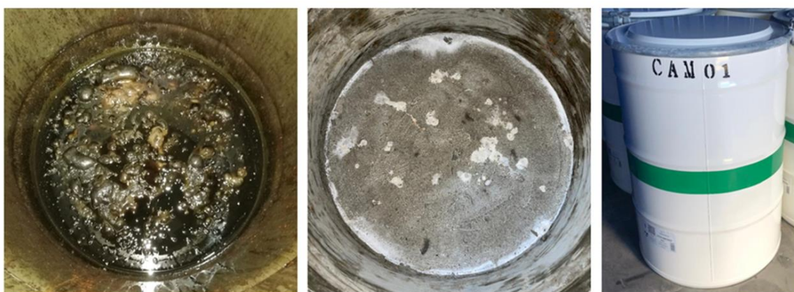
Figure 33: Real waste in the drum before (left) and after (middle) the solidification with Nochar N910 and cement inside a 220 L drum (right)
