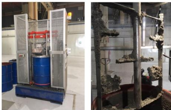
Figure 28: Full-scale solidification system (left) and removable impeller (right) [147]
