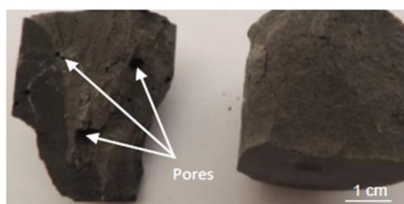
Figure 7: Samples with 40 % waste loading without (left) or without (right) addition of surfactant [19]
