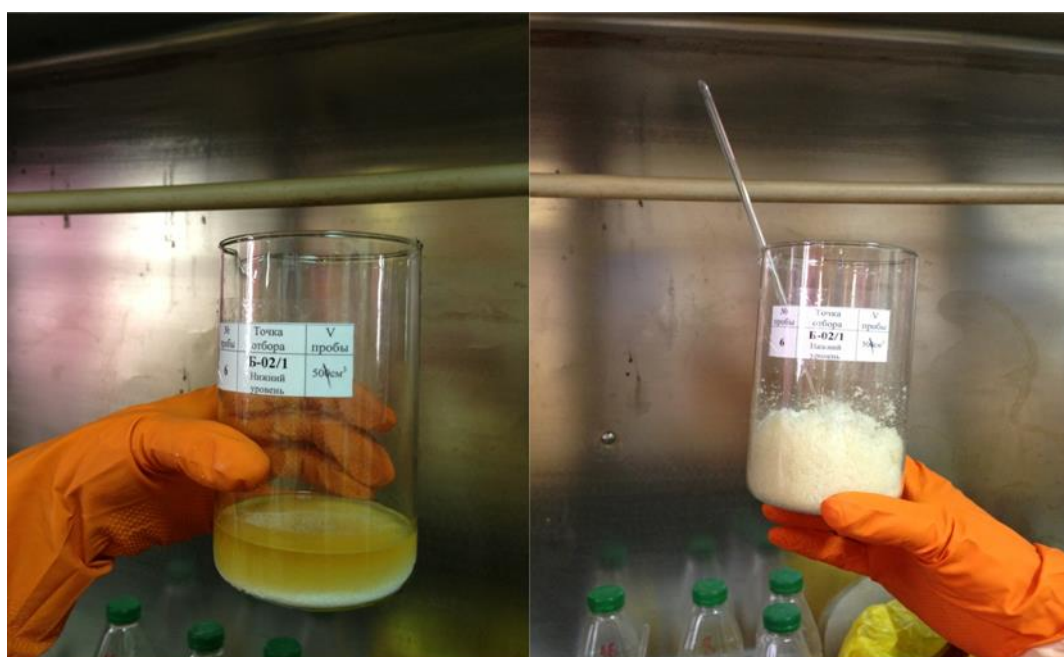
Figure 35: Sodium hydroxide in liquid form (left) and solidified sodium hydroxide with N960 at 3:1 ratio (right) [150]
