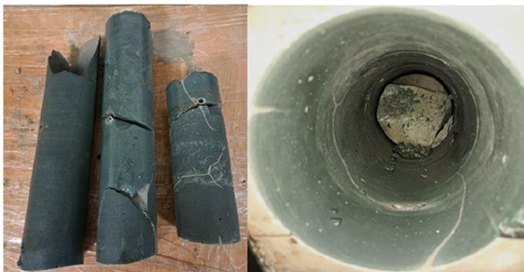
Figure 13: Core samples (left) from 100 L drum with oil waste (10 %) immobilised in MK-based GP, from the bottom, centre, and top of the drum (left to right); drilled hole (right) [19]
