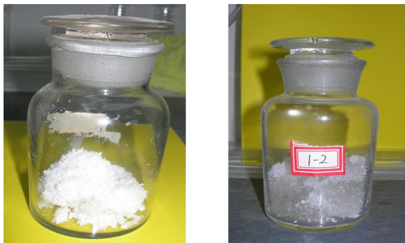
Figure 20: Solidification of TBP/OK after 6 weeks (waste/polymer ratio 1:1 (left); waste/polymer ratio 3:1 (right)) [149]
