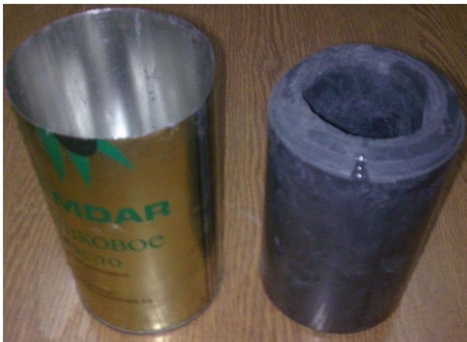
Figure 37: Sulfur composite container of laboratory scale [150]
