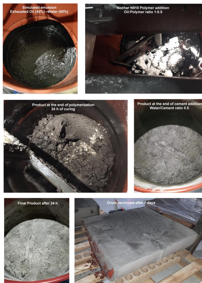
Figure 29: Full-scale trials – solidification procedure and final product [147]
