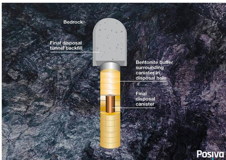
Figure 3 A canister in a deposition hole
