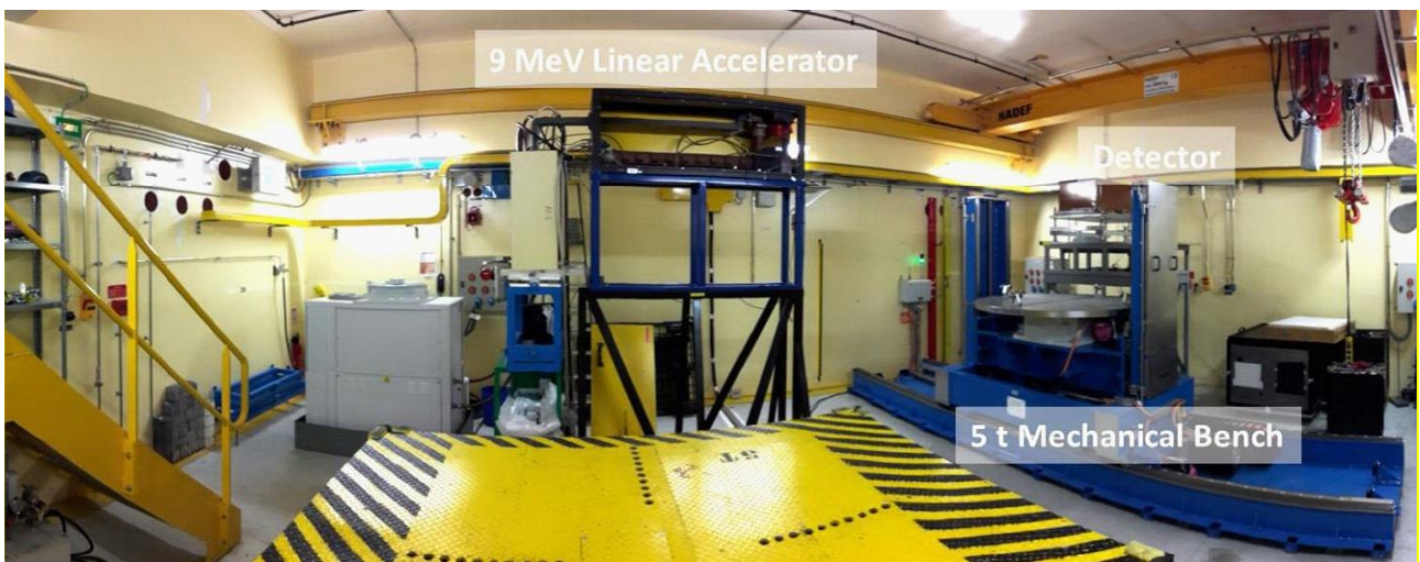
Figure 7 The CINPHONIE cell hosting a high energy photon imaging system in the CHICADE basic nuclear facility, at CEA Cadarache (Pérot et al., 2018).
