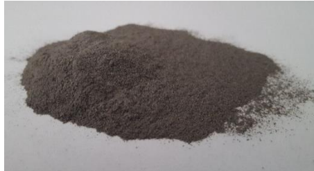
Figure 6.2. Obtained simulant ash from wood pyrolysis.
