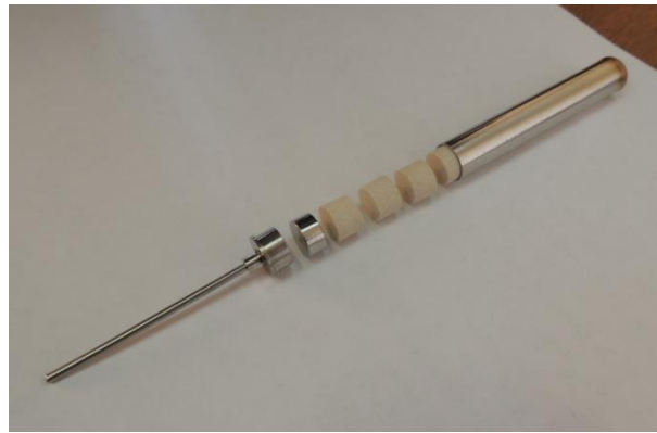
Figure 6.8. HIP canister prepared with pellets of 70% geopolymer, 30% ash.
