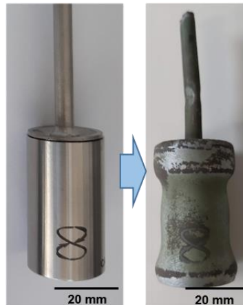
Figure 3.1. HIP canister with evacuation tub attached, before (left) and after (right) HIP processing.
