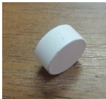
Figure 6.5. Pellet of 70% geopolymer, 30% ash after sintering at 1020 °C.
