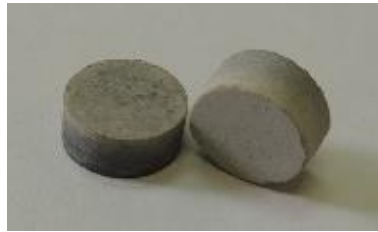
Figure 6.6. Pellets of 70% geopolymer, 30% ash after hot pressing at 920 °C.
