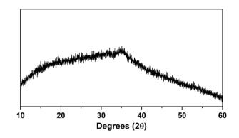
Figure 1. XRD pattern of precipitated, dried wet oxidation sludge
