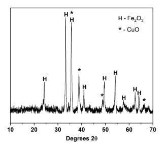
Figure 2. XRD pattern of the sludge heated to 600 °C
