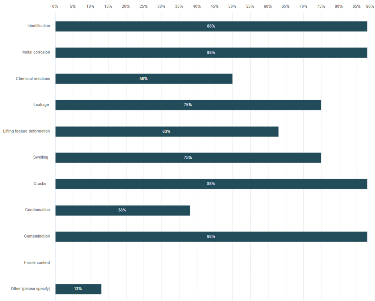
Figure 18 - Relevant parameters currently monitored on cemented waste packages
