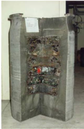
Compacted ILW solid wastes
