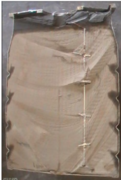
Figure 1 - Sectioning of a full-scale drum from inactive trials using simulant Dounreay Fast Reactor raffinate [16] [17]
