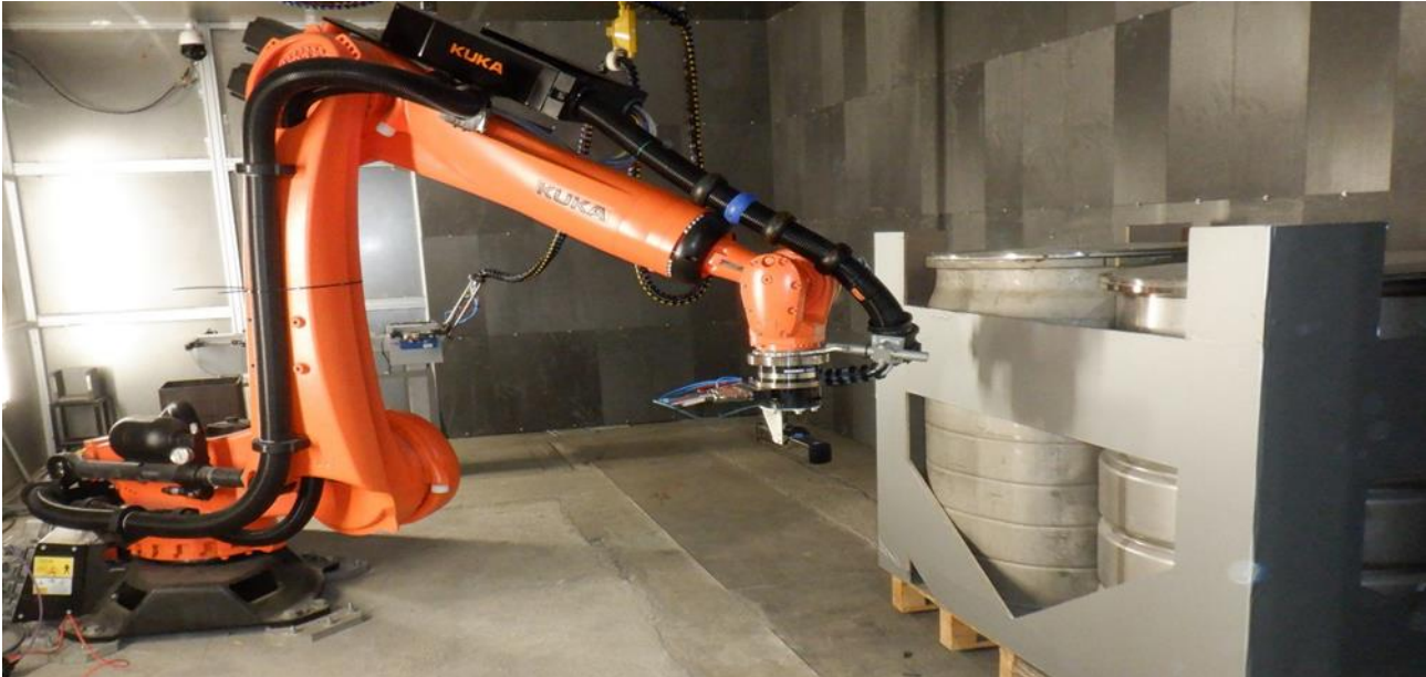
Figure 27: 500L drum being inspected by transducer mounted on industrial 6 axis robot.
