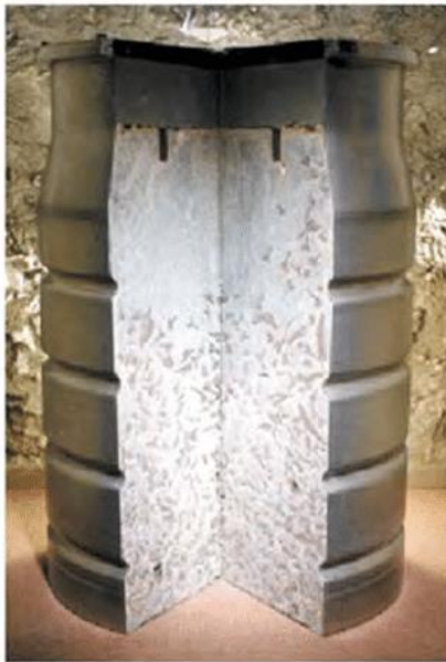
Figure 3 : Magnox package encapsulating a mixed cement matrix.
