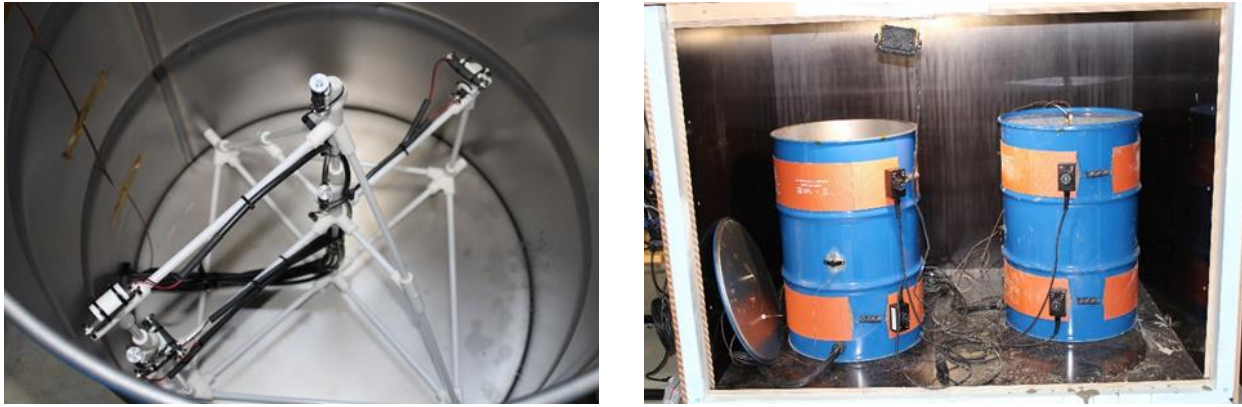
Figure 6-5 Sensor placement inside the drum (left) and two drums in the temperature chamber (right).
