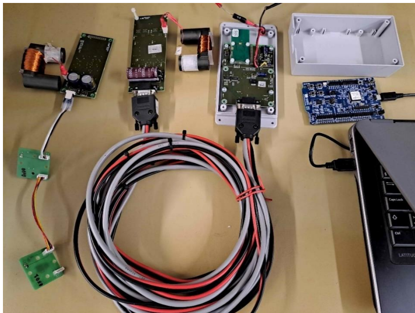
Fig. 8 Test system of the wireless link through the steel cover of the drum. The components from the left to the right are the transponder unit PCB with a connected antenna and two SensorNode PCBs, the reader unit PCB with a connected antenna, the microcontroller unit with a connection cable to the reader unit, and the laptop computer with GUI software and a Bluetooth dongle (commercial PCB) for the communication with the microcontroller unit.
