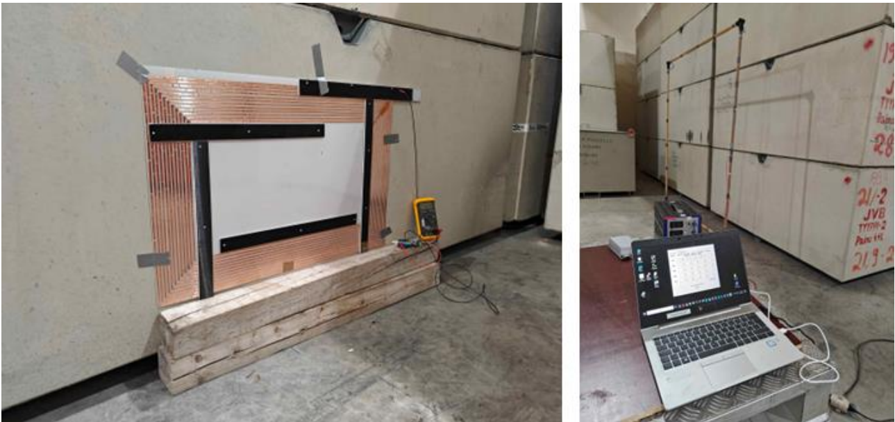
Fig. 13: Test set-up for data acquisition from the transponder unit through a concrete container.
