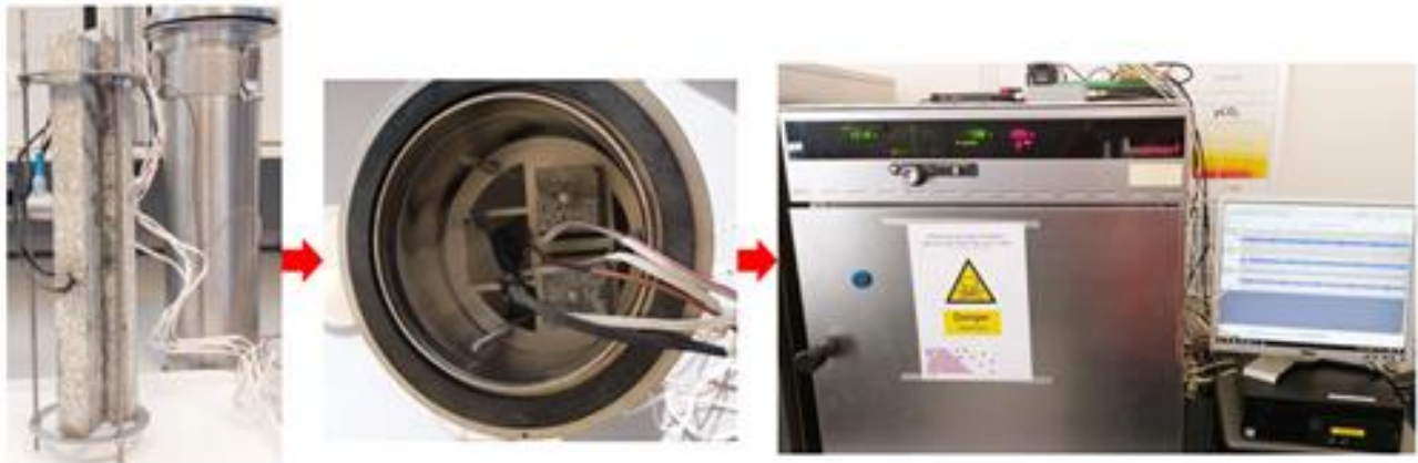
Fig. 5: Mortar bar placement in a high temperature chamber, at 80 °C, for a duration of 1 month
