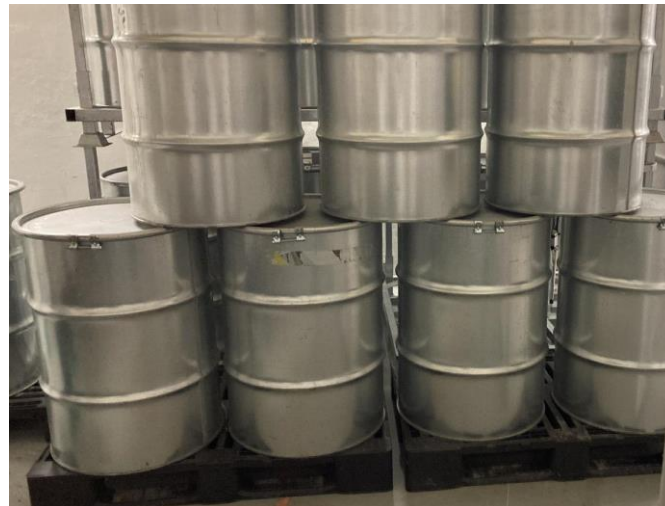
Fig. 14. The final demo configuration, the wires were disconnected and other drums filled with concrete were placed in front of the mockup.
