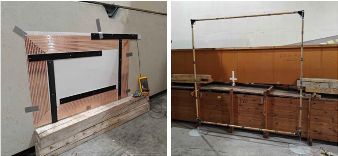
Fig. 12: Test set-up with the transponder unit antenna on the outer side of a concrete container. The leftmost photo is the transponder unit and the rightmost photo the antenna of the reader unit at the same side of the container.
