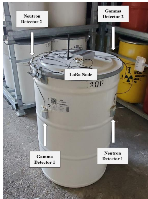
Fig. 5 LoRa node installed on a cemented 380 L overpack.
