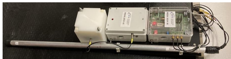
Fig.6. A complete monitoring unit consisting of one SiLiF and one SciFi detectors with the related electronics.
