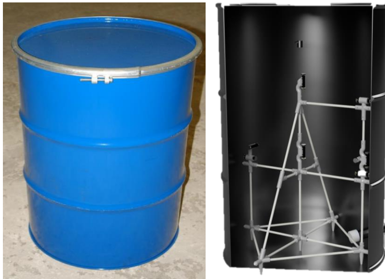
Fig. 10: Real-life barrel (left) and drawing of the supporting structure for the vibrating strain wires and thermistors (right)
