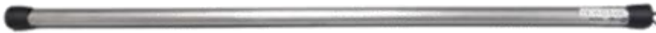
Fig.2. The SciFi detector consisting of a 3 mm diameter, 80 cm long, scintillating fiber coupled at each end to a SiPM and enclosed in an aluminium pipe.
