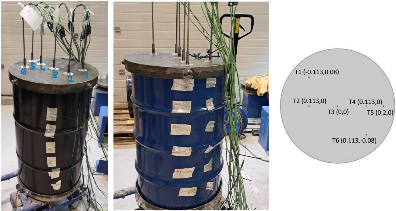
Figure 4-4: The temperature measurement setting in 100 L black drum (left), 100 L blue drum (middle) and thermocouple position in the drum lid (right).
