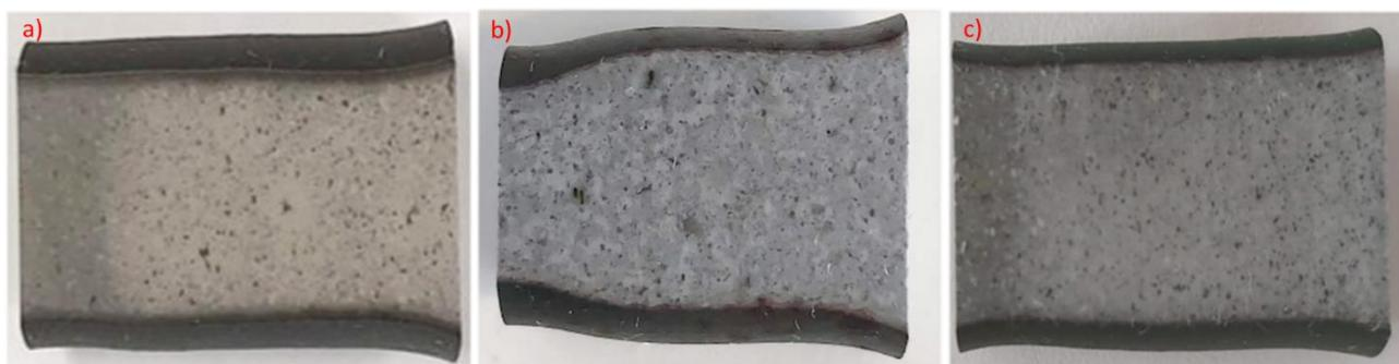
Figure 53. Photographs of HIP can cross sections of HIPed a) ground ash b) ground ash + 5 wt.% Na<sub>2</sub>B<sub>4</sub>O<sub>7</sub> and c) ground ash + 5 wt.% NaAlO<sub>2</sub>.
