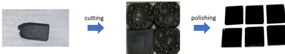
Figure 44 : Preparation of glassy samples (named V55-1).
