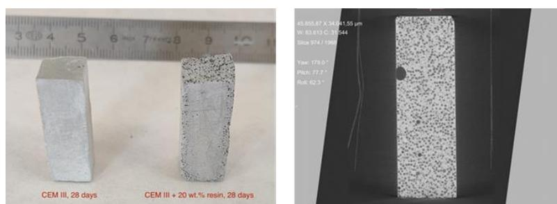
Figure 3. Prismatic specimens (1x1x6 cm) of CEM III and CEM III loaded with a 20 wt.% of thermally-treated IERs.
