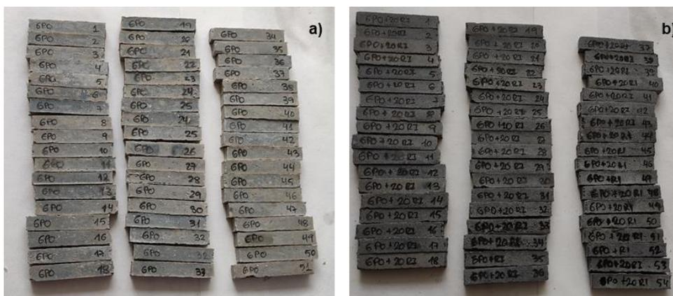
Figure 2. Geopolymer specimens (a) without and (b) with thermally-treated SIERs prepared for leaching tests conducted in Task 6.6.
