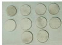
Figure 45: Preparation of pelletized ash samples (named V55-2).
