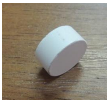
Figure 5-5. Pellet of 70% geopolymer, 30% ash after sintering at 1020 °C.
