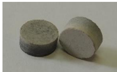
Figure 5-6. Pellets of 70% geopolymer, 30% ash after hot pressing at 920 °C.
