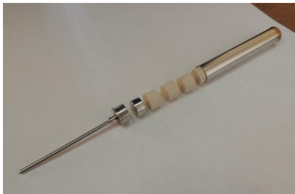
Figure 5-8. HIP canister prepared with pellets of 70% geopolymer, 30% ash.
