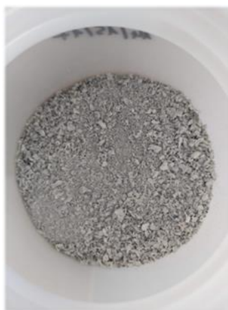
Figure 4-7. Photograph of as-received simulant IRIS ash; the inner diameter of the container is 12.5 cm.
