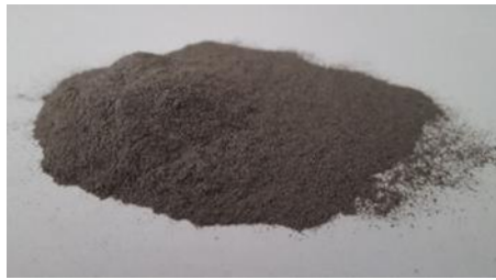
Figure 5-2. Obtained simulant ash from wood pyrolysis.
