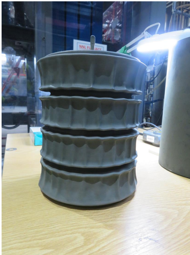
Figure 3-17. HIP can two showing well consolidated lobes which have sprung apart as the HIP pressure was released.
