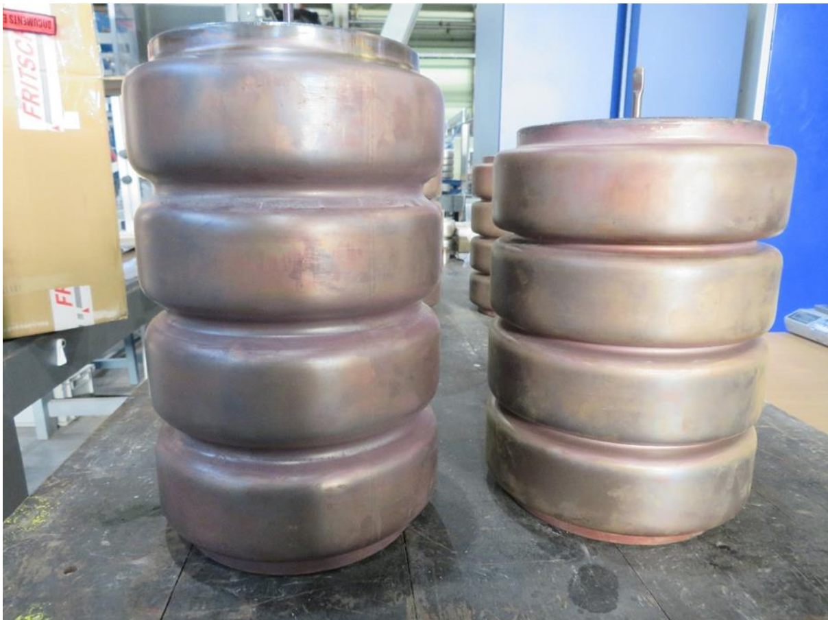
Figure 3-16. Bloated HIP can one alongside a non-deformed HIP can of identical design.
