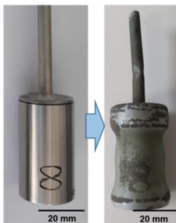
Figure 2-1. HIP canister with evacuation tub attached, before (left) and after (right) HIP processing.
