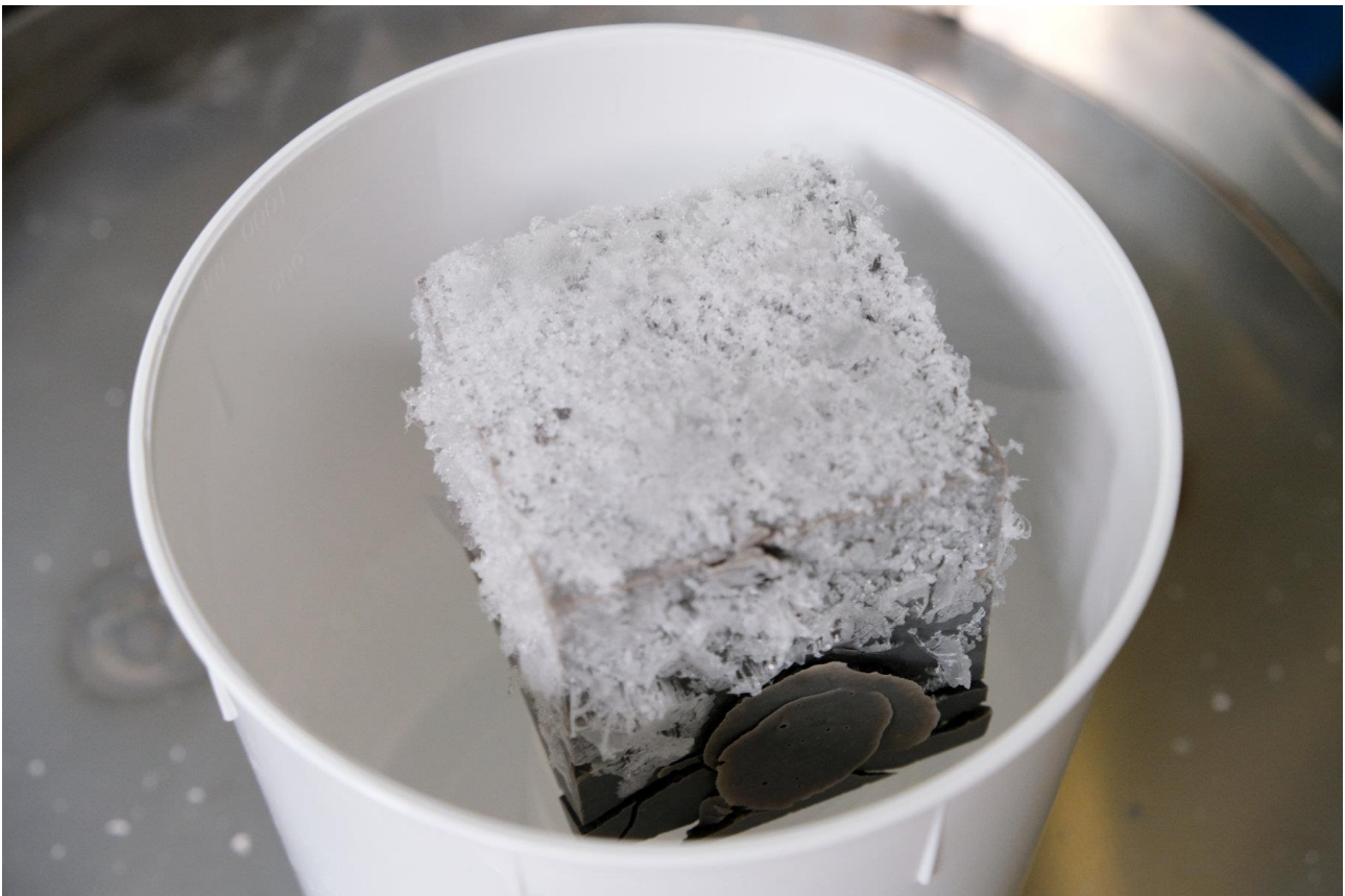
Figure 26: A cracked sample with blooming effect.
