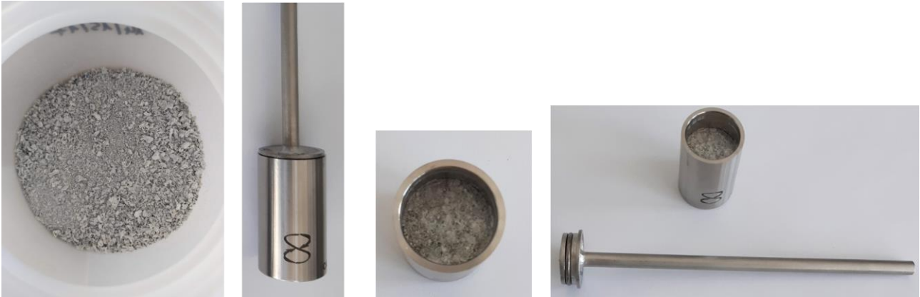
Figure 80: From left to right: Iris ashes, Empty HIP can, Packed Can with 16 g ash with a hydraulic press
