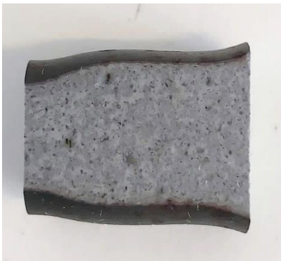
Figure 84: The inside of HIP Can ready for analysis.
