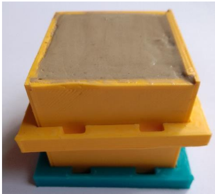
Figure 96: Geopolymer matrix samples (cubes moulds of the 5x5x5 cm side)
