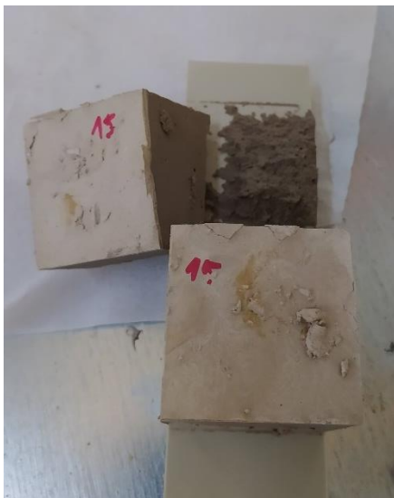
Figure 31: The broken samples during demoulding process (left) and not completely solid samples before Compressive testing (right)
