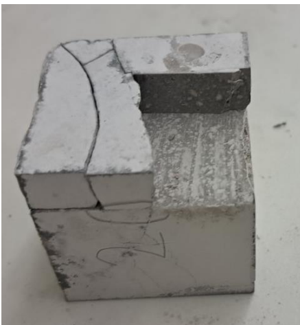
Figure 17: The blooming effect of the LK10 geopolymer with 20 w.% of waste loads. All surface is covered with the blooms of sodium carbonate hydrates.
