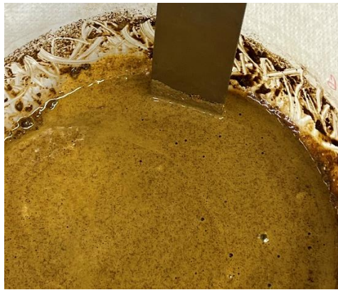
Figure 69: Sludge obtained downstream of the Fenton-like wet oxidation process.
