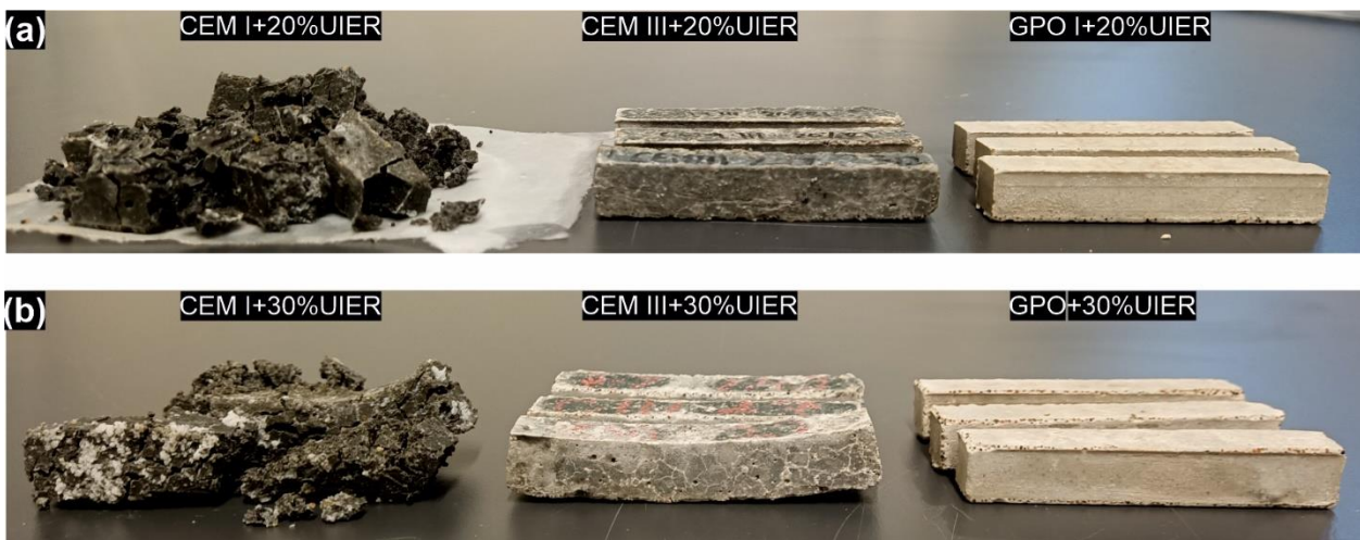
Figure 52. Visual aspect of paste samples with (a) 20%UIER and (b) 30%UIER after 3 months at 21°C and 99%RH
