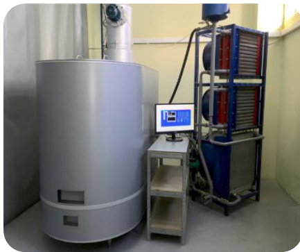
Figure 19. System for thermal treatment based on gasification technology.
