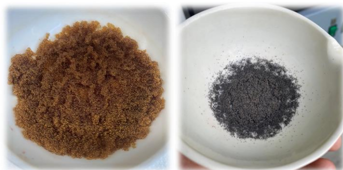
Figure 12. Spent cation-exchange resins: (left) before treatment; (right) after treatment.
