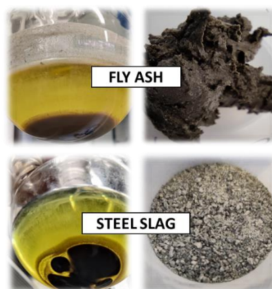
Figure 18. Liquors and residues downstream of wet oxidation process by using fly ash (top) and steel slag (bottom) as a catalyst.
