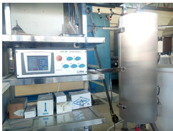
Figure 3. Laboratory-scale drop tube reactor in CIEMAT.
