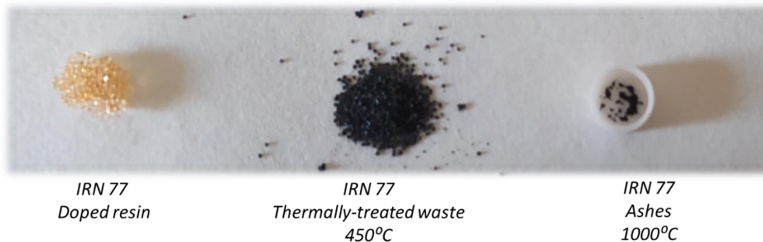
Figure 6. Photo of IRN77 and IRN78, thermally treated waste obtained at 450°C and residue obtained in the crucible after the thermobalance tests (up to 1000°C).
