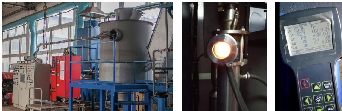
Figure 25. System for thermal treatment of the radioactive wastes based on gasification technology with a plasma reactor.
