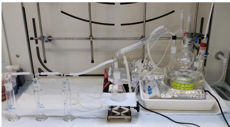
Figure 14. Experimental set-up of a Fenton-like wet oxidation process at intermediate laboratory scale (up to 200 g of resin).
