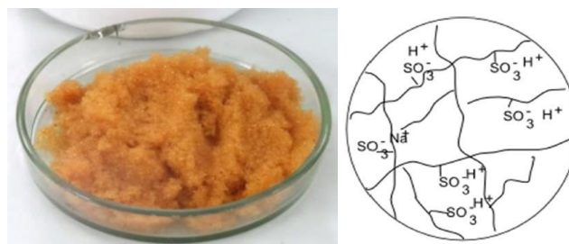
Figure 27. Chemical structure of the strong acidic cationic ion exchange resins with functional groups of -\text{SO}_3\text{H}^+ .
