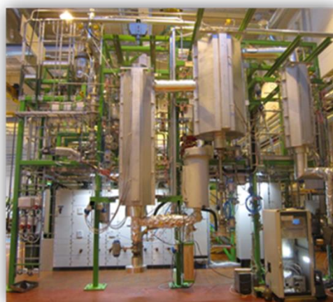
Figure 34. Bench-scale atmospheric-pressure gasification test rig (BFB100).
