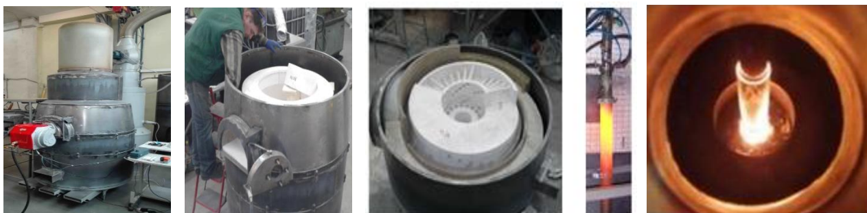
Figure 22. The installation trials of plasma torch gasification.
