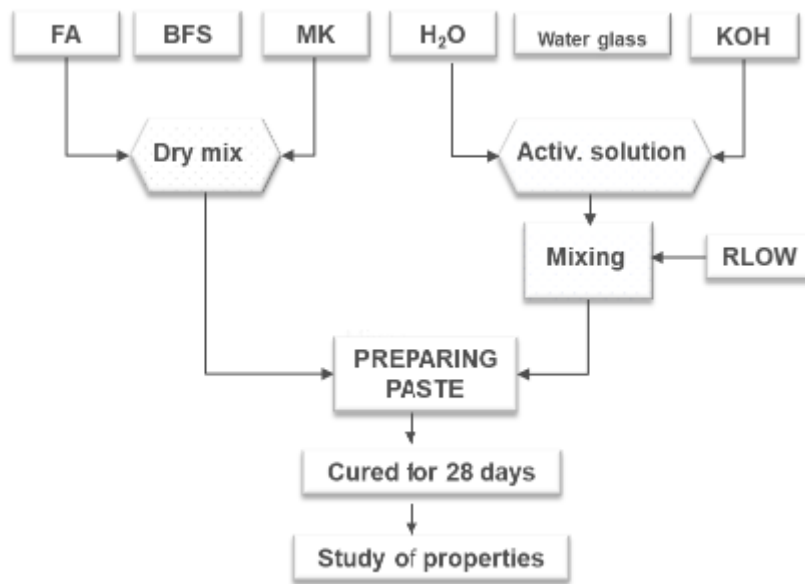
Figure 4: Process flow diagram for the preparation of a MIX-based wasteform
