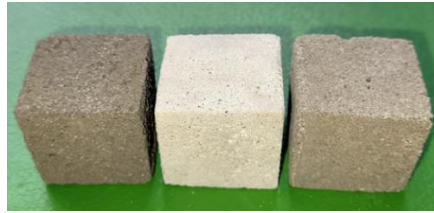
Figure 4. Specimens after 1 year of aging in distilled water, from left to right: MKPC - FA, MKPC – BFS and MKPC – FA - BFS.
