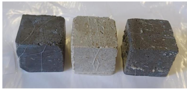
Figure 8. MKPC - FA, MKPC - BFS and MKPC – FA - BFS specimens (from left to right) after leaching in an alkaline solution for 90 days.
