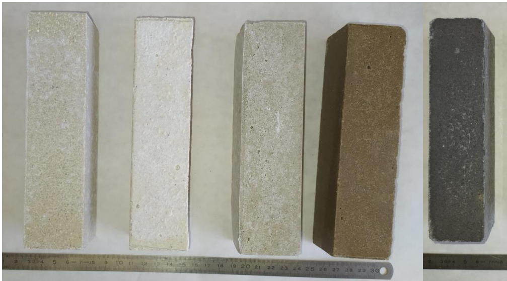
Figure 1. Visual aspect of MKPC mortars containing (from left to right): metakaolin A, metakaolin B, wollastonite, pumice and volcanic ash.
