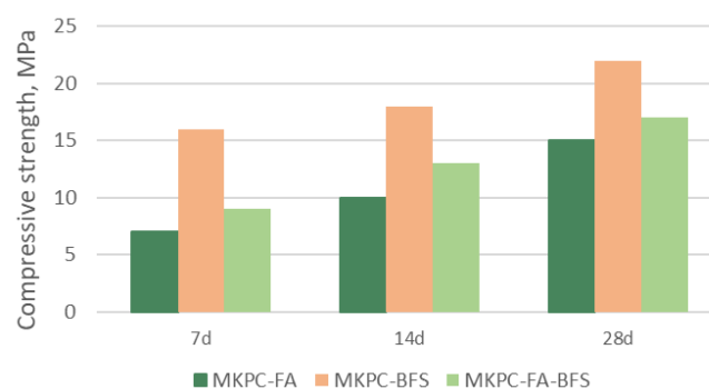
Figure 49. The compressive strength of MKPC based samples.
