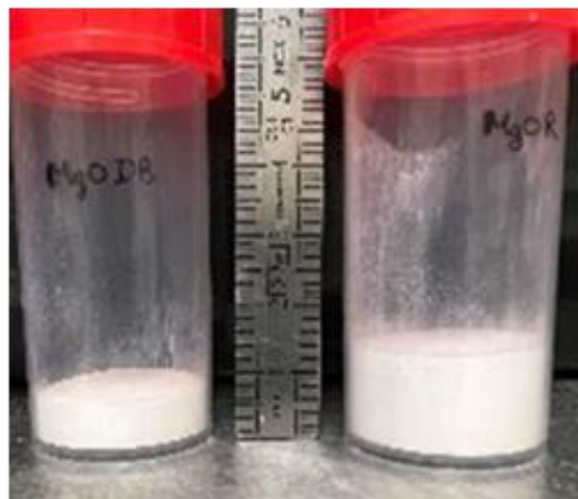
Figure 31. Equal mass of reactive MgO and DB MgO.
