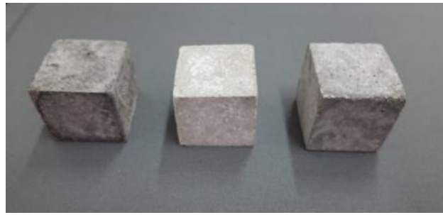
Figure 45. Samples (3x3x3 cm) of MKPC-FA, MKPC-BFS and MKPC-FA-BFS (from left to right).
