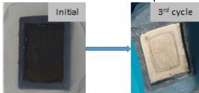
C. Evolution of sample treated at high concentrations (15mM KMnO 4 and 18.5mM H 2 C 2 O 4 )
