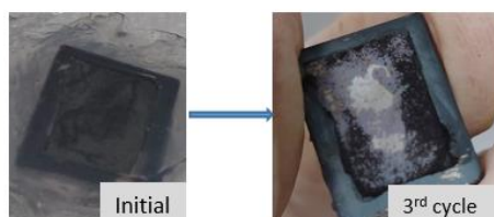
Figure 17 Evolution of the sample after 3 cycles of the HP oxidation during COREMIX process (15mM \text{HMnO}_4 followed by 18.5mM \text{H}_2\text{C}_2\text{O}_4 ), applied at 80°C for 3 hours/step
