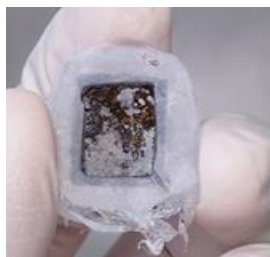
Figure 19 Black precipitate on sample following application of the COREMIX loop with UV light with 15mM KMnO_4 in 3mM HNO_3 followed by 18.5mM oxalic acid, heated up to 95°C in the reservoir
