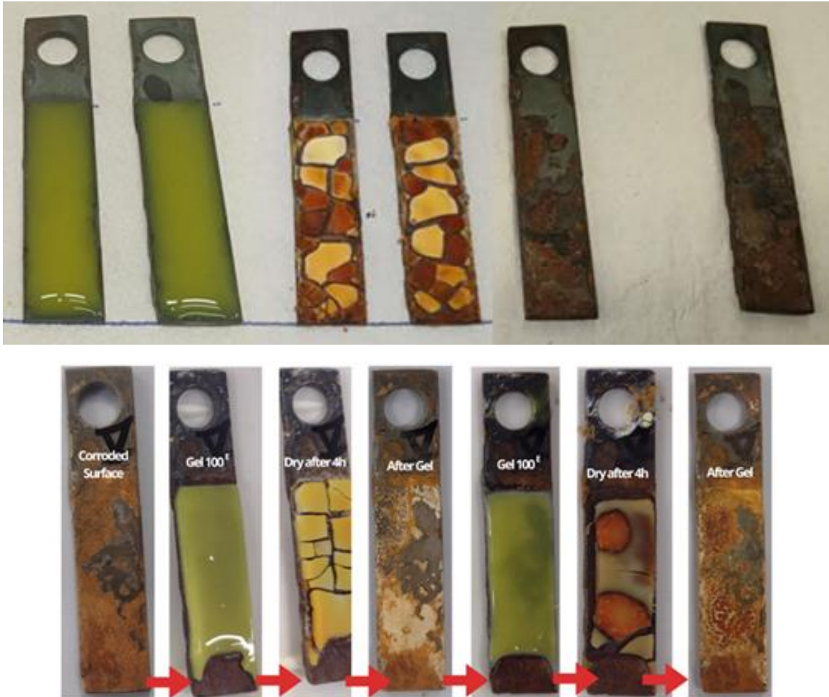
Figure 8. Decontamination of strongly oxidized SS samples by Aspigel 100E: one application (top), and successive applications (down).
