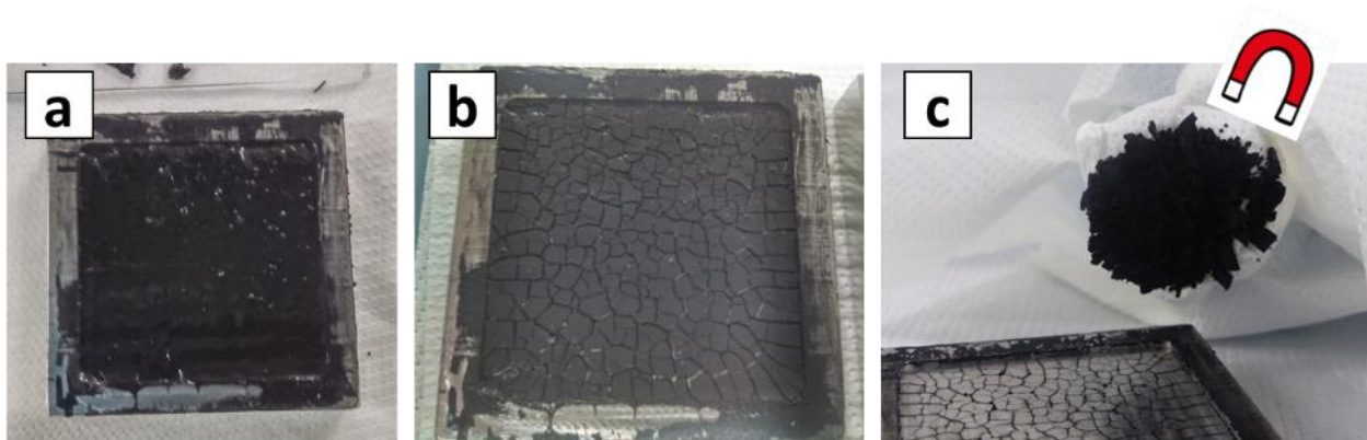
Figure 36. Millimeter layer of Gel_3 (left), formation of solid residues after drying (center) and attraction of the solid residues by a magnet (right).
