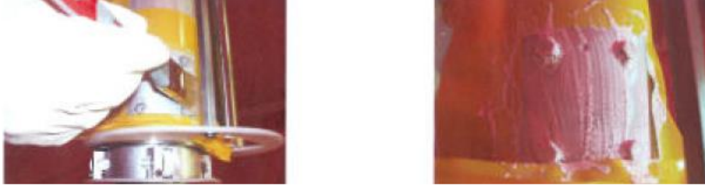
Figure 4: Decontamination of an aluminium slave arm
