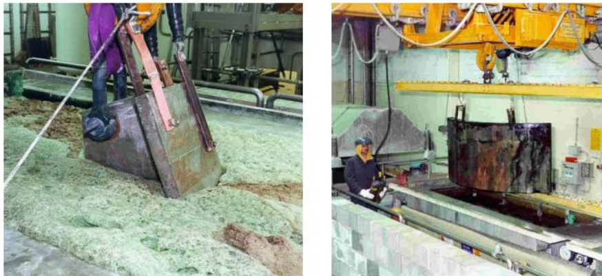
Figure 1: Before (left) and after (right) images of stainless steel being decontaminated in an acid bath [1].
