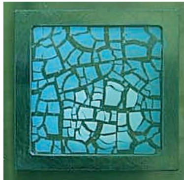
Figure 1: Example of millimetric pieces generated by drying of the gel during decontamination [3]
