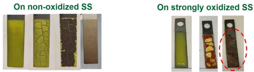
Figure 3: Examples of decontamination gel application and resulting surface appearance on non-oxidised and strongly-oxidised 316L stainless steel (Gossard, CEA) [4].
