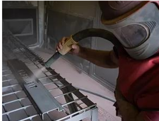
Figure 1: Dry abrasive blasting [3]
