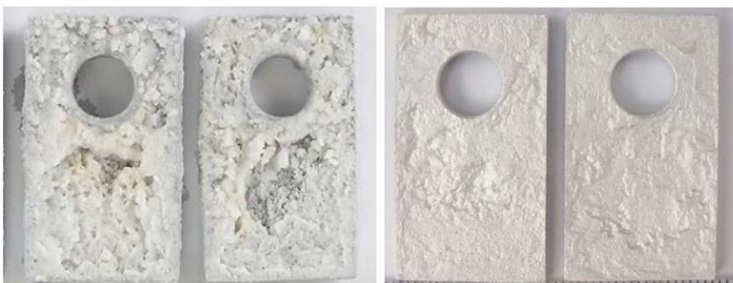
Figure 16. Aluminium surfaces after exposure to synthetic water HORMISEC
