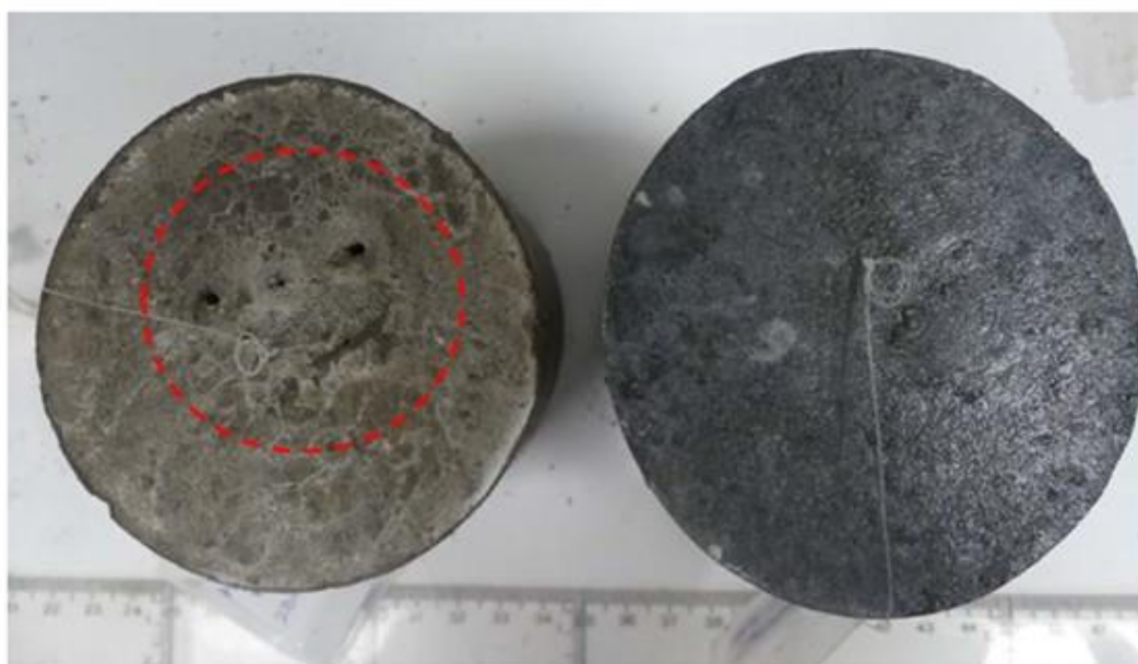
Figure 35. Comparison between CABRIL (left) and MPC (right) mortar specimens with embedded Al. Holes from H 2 release in CABRIL mortar are appreciated (red circle)
