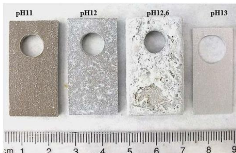
Figure 19. Aluminium surfaces after 720 hours exposure to \text{Ca}(\text{OH})_2 solutions at different pH
