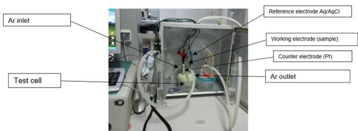
Figure 6. Electrochemical test cell assembly (in solution systems)
