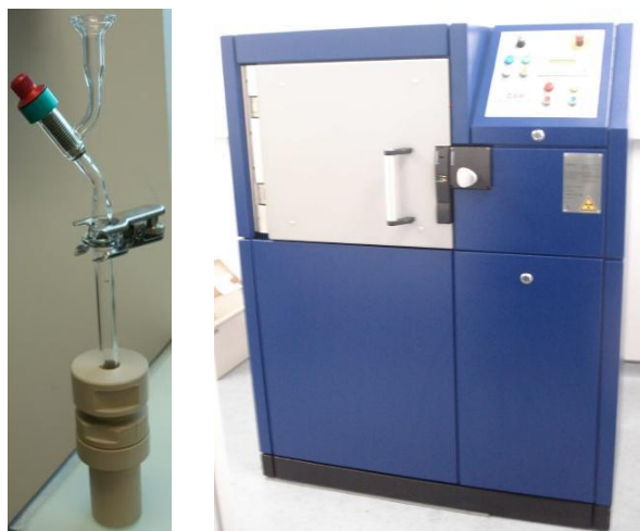
Figure 2: PEEK cell (left) and the gamma irradiator with Cs-137 radioactive source (right).
