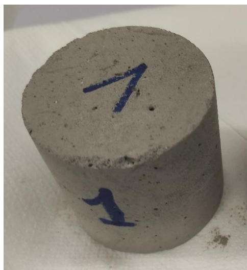
Figure 14: MPC sample at the end of the 90-days leaching test
