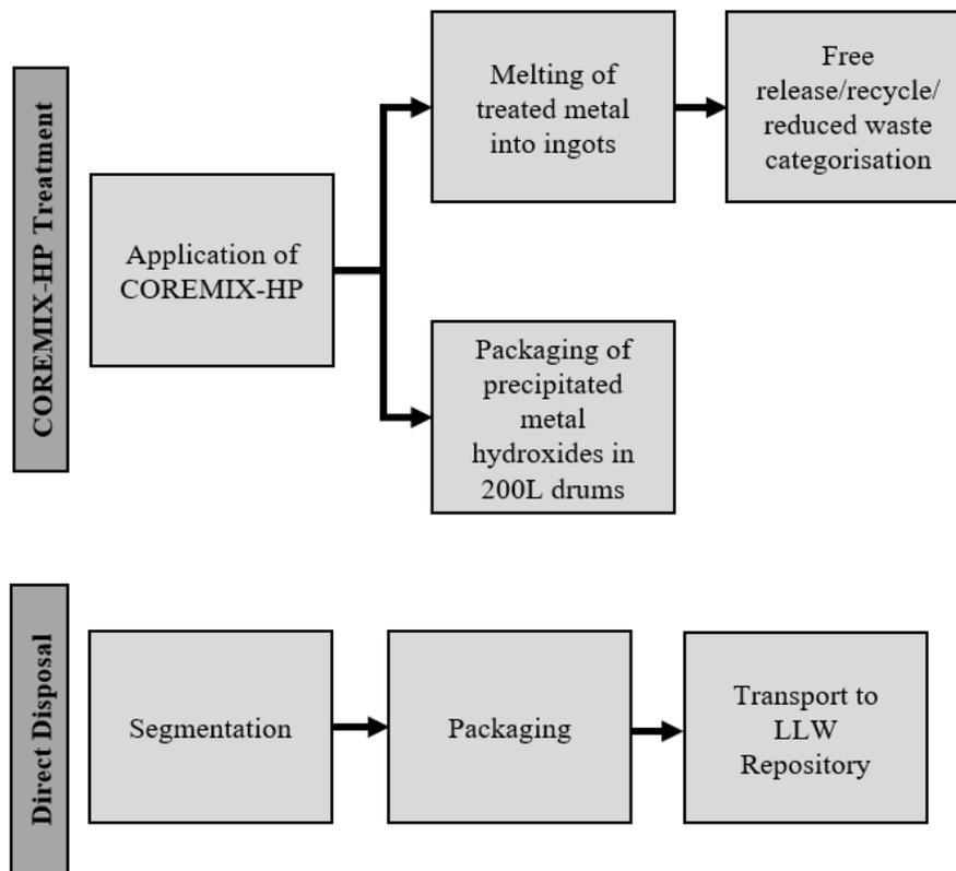
Figure 3: Steam generator treatment options considered in this study using COREMIX-HP
