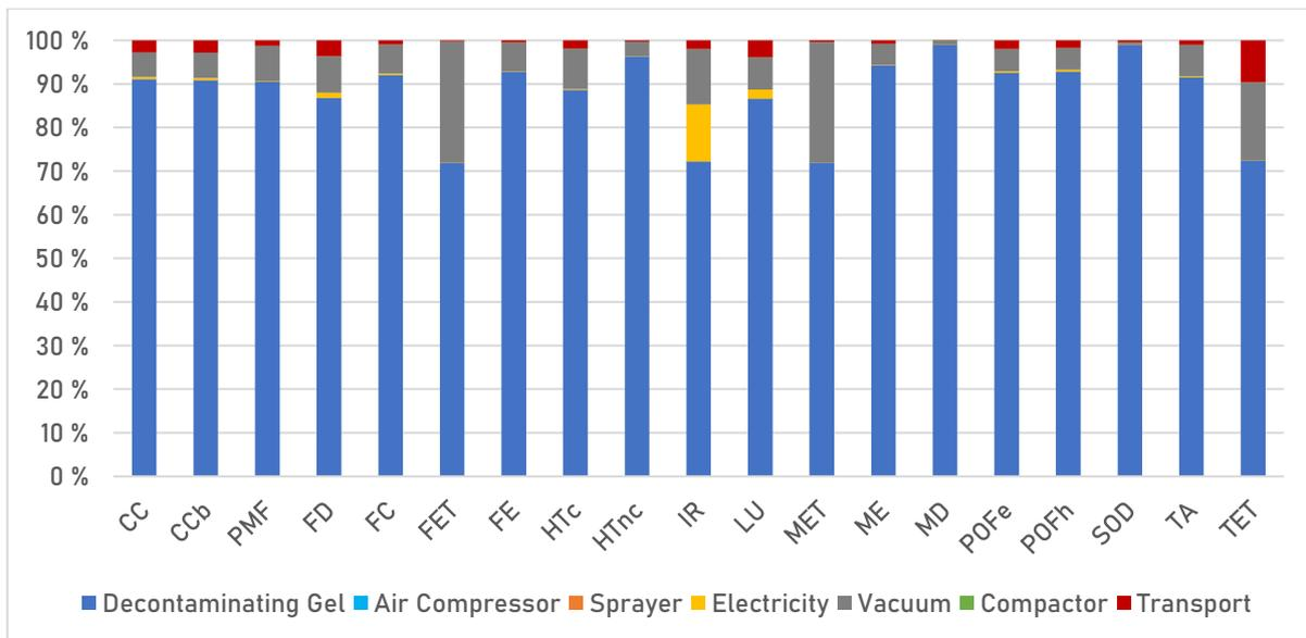
Figure 6: Impacts of using gel decontamination on a hot cell
