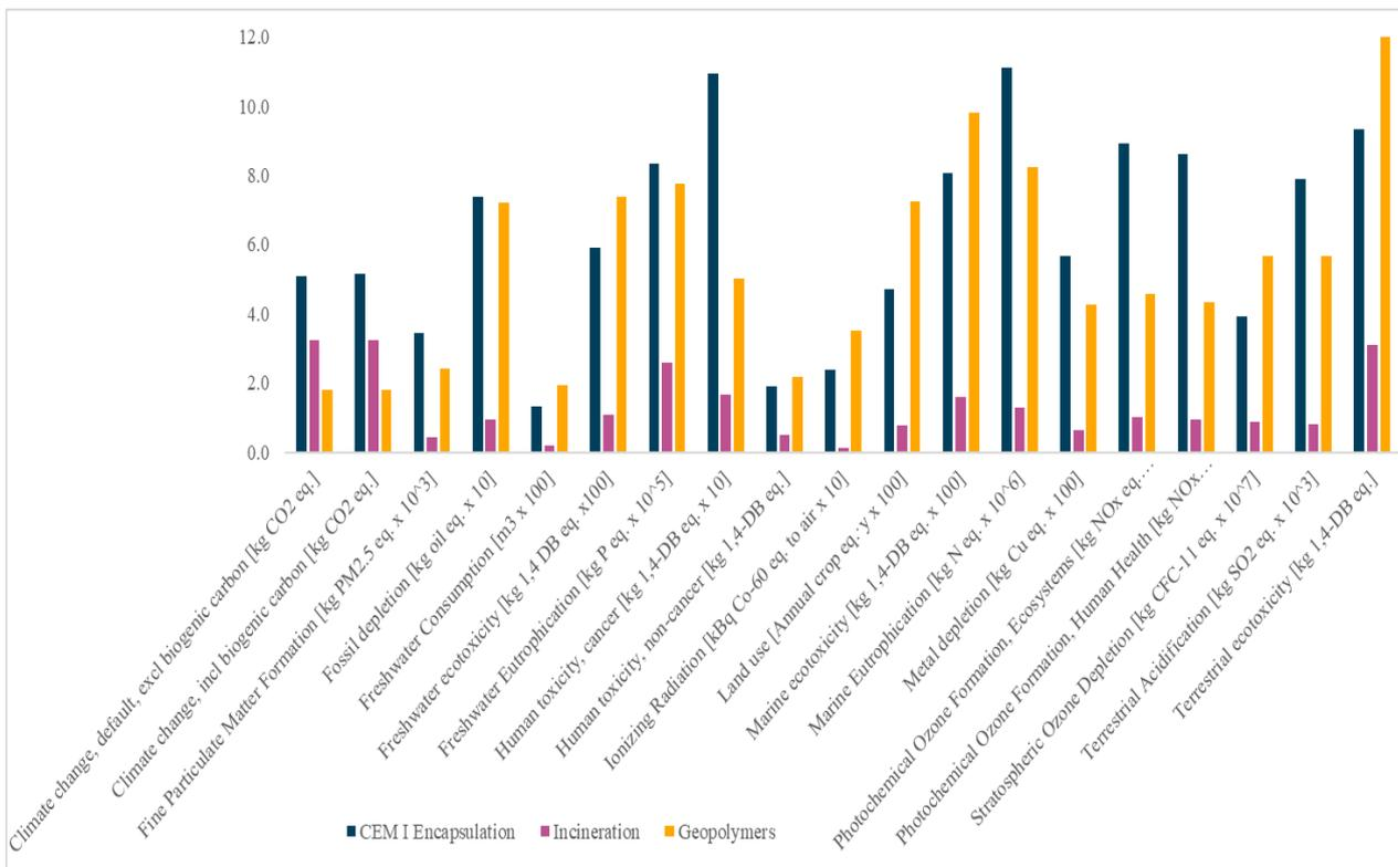
Figure 8: Life cycle environmental impacts of incineration, cementation and geopolymer encapsulation
