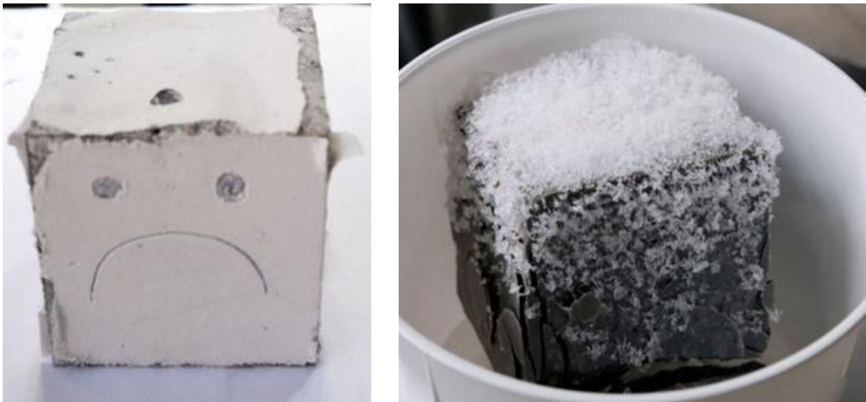
Figure 3. Blooming effect on prepared metakaolin sample (left) and blooming effect on the cracked sample with 25 wt.% in high moisture environment (right).
