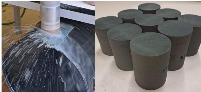
Figure 3. Wet curing of 100 L drum and extracted samples before compressive strength analysis.
