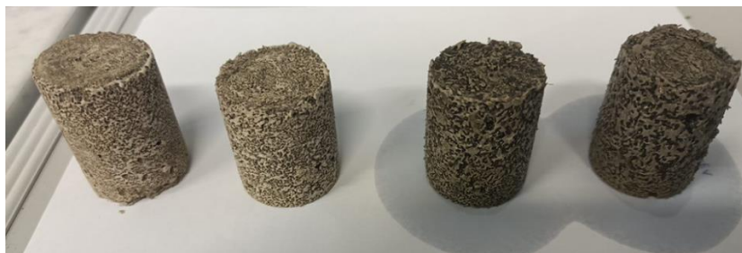
Figure 2. Samples containing increasing amounts of TBP/dodecane prepared via pre-absorption on NOCHAR N910 (mass ratios from 3:1 to 6:1, constant waste loading of 30 vol%). Large cavities are visible due to the difficulties in homogenizing the paste with the absorbed waste.
