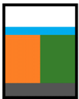
Figure 5 - Qualitative scheme of specimen composition. 1 part OPC [gray], 0.6 parts water [blue] and 3 parts sand [orange], replaced at 50% by volume with rPU [green]
