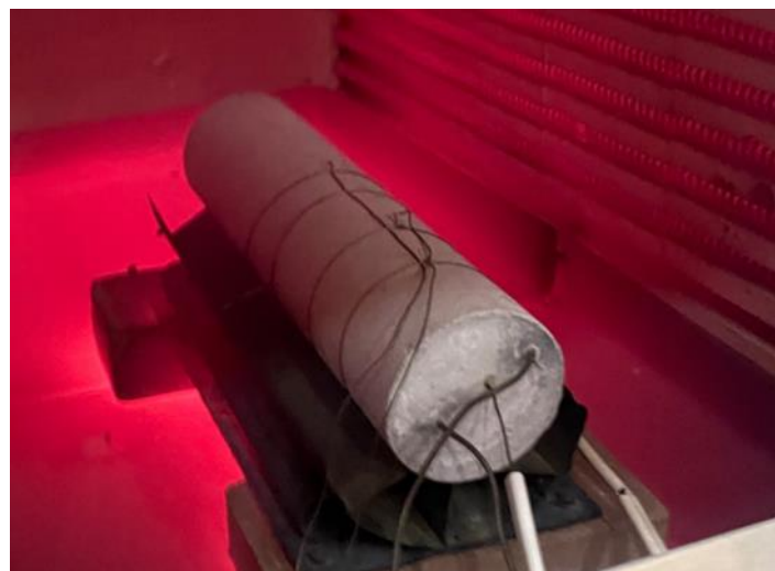
Figure 53. T5.4.7 Thermal conductivity trends with linear interpolation for (un)aged (a) concrete. In b) image from thermal test execution on RLOWs simulant/concrete.
