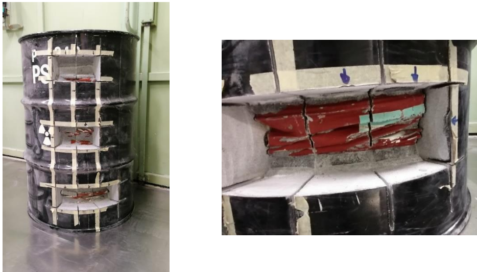
Figure 104. Cemented LLW drum considered for the characterization within this study. Samples were taken at PSI from upper, middle and bottom positions.
