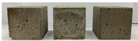
c) Geopolymer samples containing rPU previously pre-impregnated with 10, 10, and 20 %wt. of UG-LSC.
