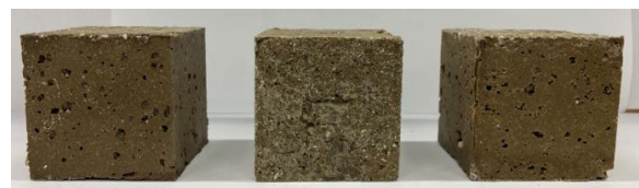
b) Geopolymer samples containing rPU previously pre-impregnated with 10, 10, and 20 %wt. of TBP-k.
