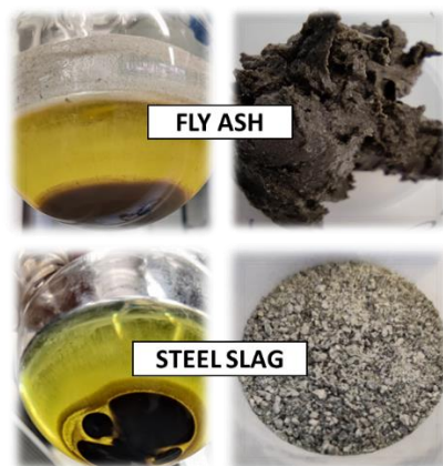
Figure 92. Liquors and residues downstream of wet oxidation process by using fly ash (top) and steel slag (bottom) as a catalyst.
