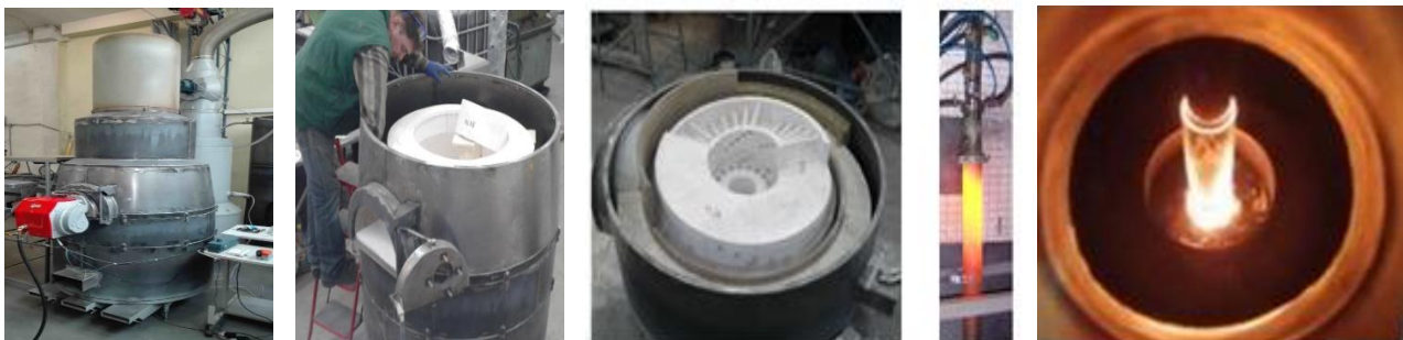
Figure 65. The installation trials of plasma torch gasification.
