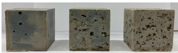
a) Geopolymer samples containing 0, 5, and 10 %wt. of rPU.
