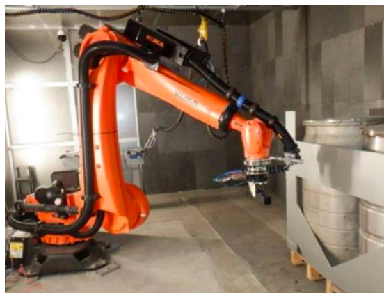
Figure 110. NNL feasibility trial of stitching laser scanning.
