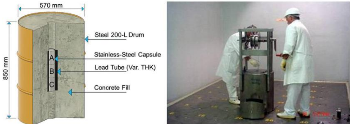
Figure 4. Potential storage solutions for the DSRSs. Left: cross section of a shielded drum [22], right: lowering source into a well type DSRS storage in Püspökszilágy, Hungary.
