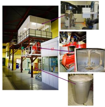
In-line mixing using a high shear mixer – STEMA platform
