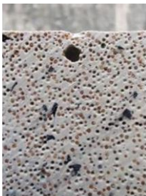
Encapsulation of ion exchange resins in a cement matrix
