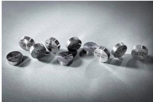
Certified reference materials EURM-800 and EURM-801 ^{60}\text{Co} in steel disks
