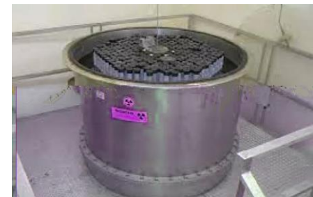
AUTH Subcritical Pile
