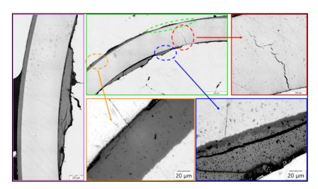
Figure 40 – Optical observations of the cladding (green and pink) and selected areas of crack (red), external zirconia (orange) and pellet/cladding interface (blue).
