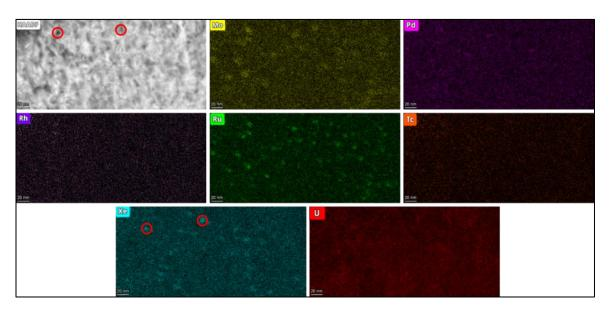
Figure 59 – EDX maps of Mo, Pd, Rh, Ru, Tc, Xe and U in the grain G1 of the restructured area (in at.%).
