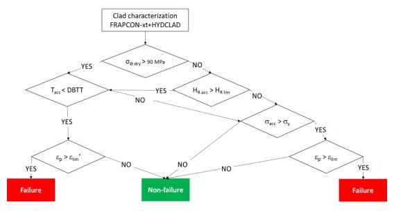
Figure 27 - Failure criteria.
