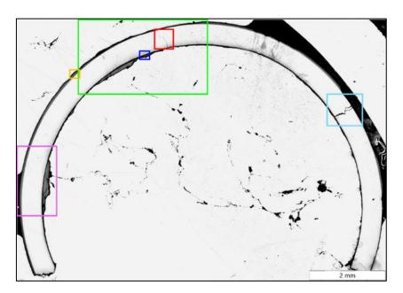
Figure 39 – Optical observation of the cladding segment and positions of the detailed areas.
