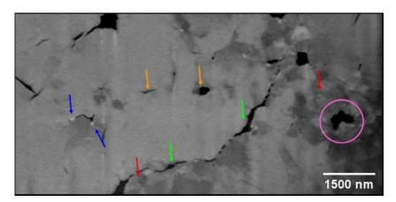
Figure 47 – SEM observation at 0.2R taken during a 3D acquisition, revealing the presence of precipitates, intragranular and intergranular bubbles and subdivided grains.
