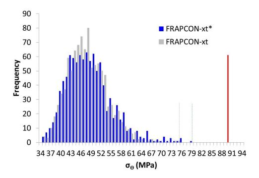
Figure 31 – Cladding hoop stresses at the dry storage onset. Predictions with FRAPCON-xt (MASSIH) and FRAPCON-xt\* (calibrated FRAPFGR).
