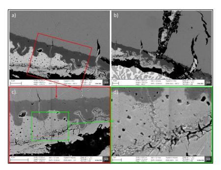
Figure 44 – SEM observations of different areas of fuel/cladding interface.
