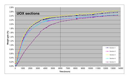
Figure 36 – Weight gain of UOx sections as a function of time.
