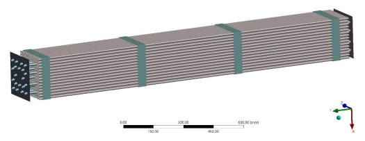
Figure 15 – FEM of a 15x15 spent-fuel sub-assembly. The model consists of 205 fuel rods, 20 guide tubes, 4 spacer grids and 1 top and bottom end piece respectively.
