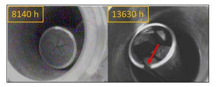
Figure 37 – Section of interest section after 8140 and 13630 h of oxidation test under air at 200 °C [5].
