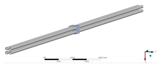
Figure 11 – Assembly consisting of four beams with an annular cylinder cross-section and a 2x2 spacer grid modelled using shell elements.
