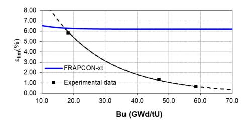
Figure 26 – Comparison of the strain limits between FRAPCON and data provided from the project.
