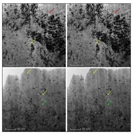
Figure 58 – TEM images of bubbles (examples indicated by yellow arrows), bubbles network (green arrow) and grain boundary (red arrow), in over-focused on the left ( $f = +1 \mu m$ ) and under-focused condition on the right ( $f = -1 \mu m$ ).
