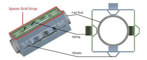
Figure 8 – Shape of spacer grid springs and dimples on an actual cladding (left: 3D view, right: lengthwise cross-section).
