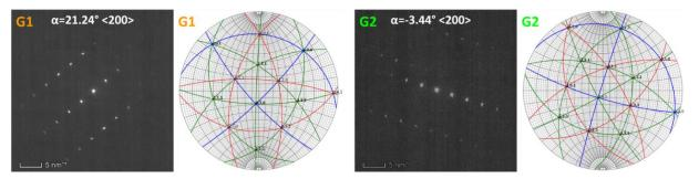
Figure 60 – Examples of diffraction patterns obtained for the grains G1 (up) and G2 (bottom) and resulting stereographic representations.
