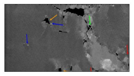
Figure 52 – SEM observation at 0.8R taken during a 3D acquisition, revealing the presence of precipitates, intragranual and intergranular bubbles and subdivided grains.
