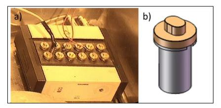
Figure 35 – (a) Oven used for long term oxidation cells, consisting of 12 cylindrical cells in a copper block and (b) example of a container, both used in the hot cell.
