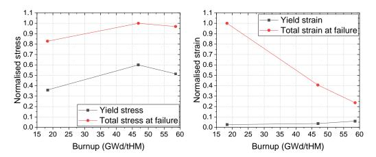
Figure 6 – Comparison of normalised stress (left) and strain (right) values at yield and at failure for different BU values.
