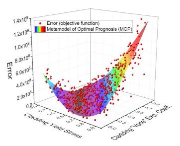
Figure 4 – Example of a MOP produced during the optimisation process. The error of each simulation is plotted against the most important parameters of the optimisation process (in this case  $\sigma$ 0 and Rinf). The best fit of each parameter corresponds to the simulation with the lowest error value.
