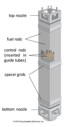
Figure 7 – Overview of basic components of a PWR fuel assembly. Original received from Encyclopaedia Britannica, Inc. [6].
