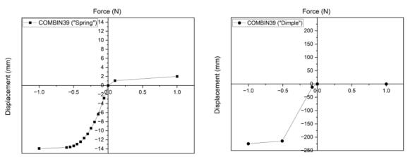
Figure 10 – Force-displacement curves describing the behaviour of springs (left side) and dimples (right side). This data is based on the report of Adkins et al. [7] and is used in the current FEM.
