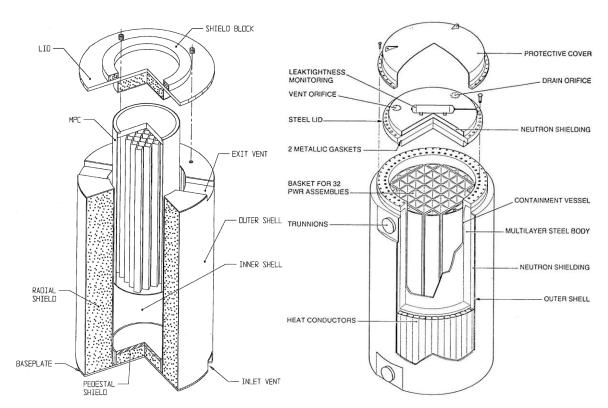
Figure 1 - MPC + Overpack / Bare Fuel Cask DSS examples from NUREG -2214 (NRC, 2019)
