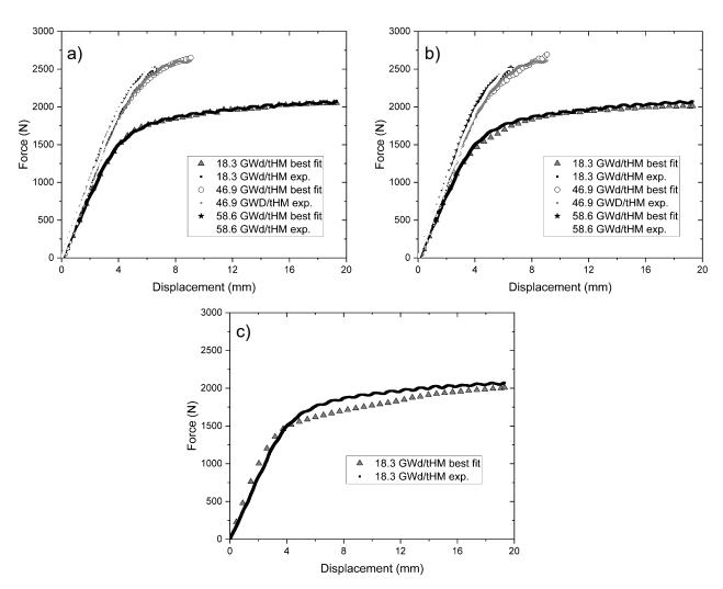
Figure 5 – Comparison between experimental force-displacement curves and best-fit curves of the 1D beam models, as derived from the optimisation process. a) Annular cylinder model, b) Cylinder model, c) Combined model.
