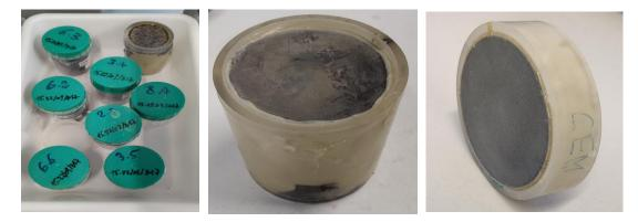
Figure 3-18: Left: Original samples received from **[ANDRA]**; Middle: the cement sample (5 cm length) that was fitted in a PMMA cylinder; Right: the cut and polished cement sample with 1 cm length.
