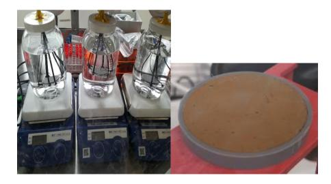
Figure 3-4: Leaching set-up of the 6 mm cement discs used by [SCK CEN].
