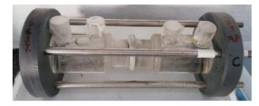
Figure 3-20: Natural diffusion set-up performed at [CSIC].
