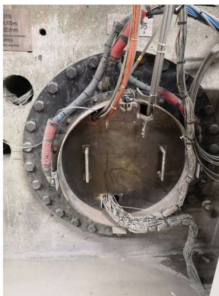
Figure 7.7: Closing plate at the head of the ALC1605 cell
