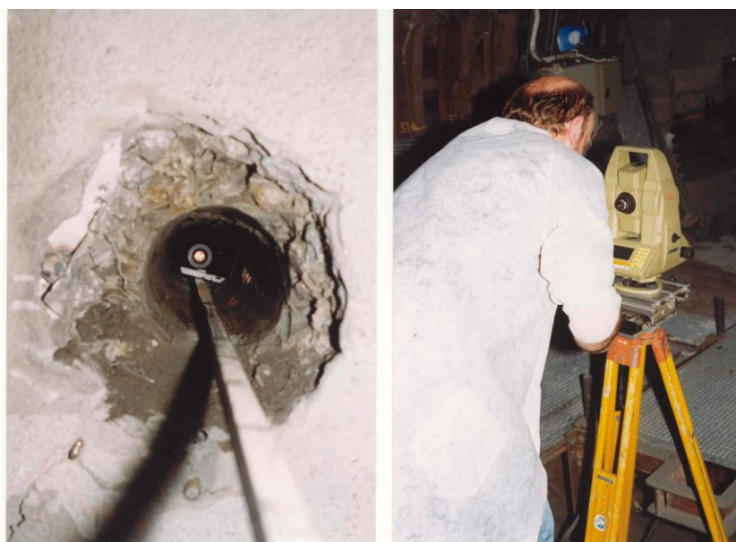
Figure 2.9 - Images showing the optical surveying of boreholes in the HADES URL [19].
