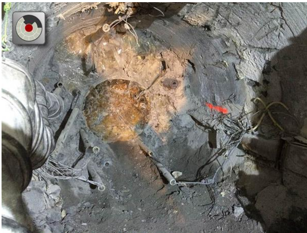
Figure 2.6 - Image of the FEBEX experimental set-up during dismantling [43].
