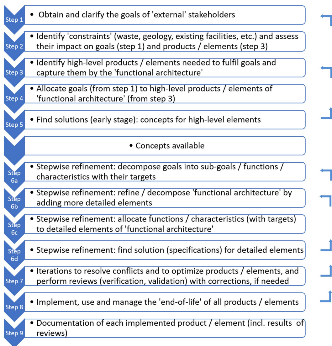
Figure 4 Overview on the different steps of requirements management to fully define the waste management system, with all the stages of the life-cycle of its elements. This process is performed in an interactive manner, as indicated by the arrows
