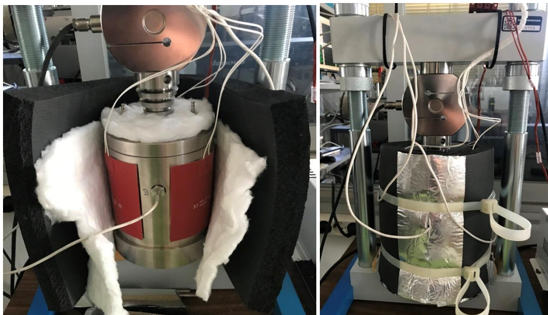
Figure 2-6. Isothermal cell wrapped in the heating mat and isolating material (left) and placed in the frame with load cell on top (right)
