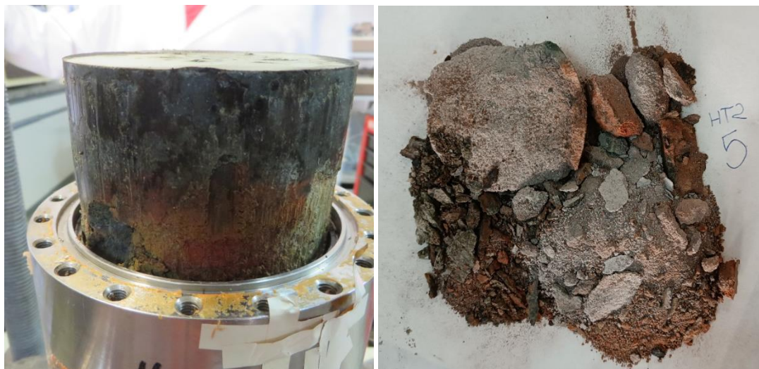
Figure 2-16. Upper part of the block from cell HT2 and material corresponding to the section closest to the heater
