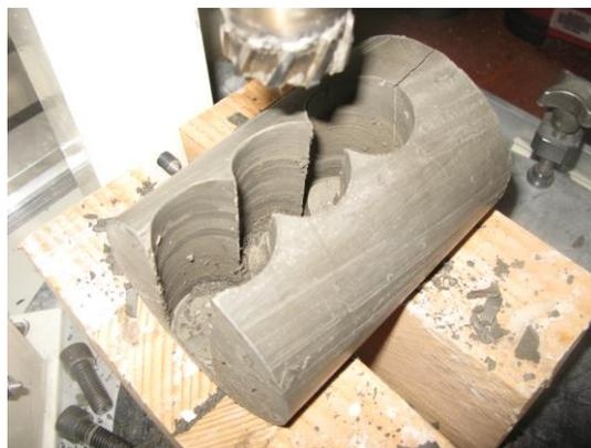
Figure 1 - Over-coring of Boom Clay with special coring tool.
