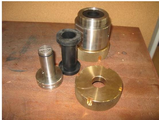
*Figure 2 - HOEK-type triaxial cell used for the creep experiments.*
