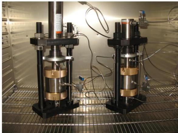
*Figure 3 - Testing bench with two HOEK-type triaxial cells and loadframe inside the oven.*
