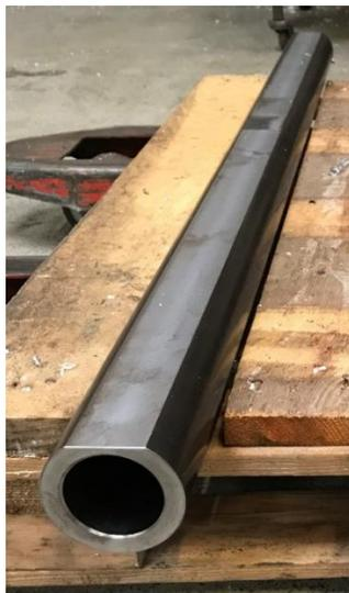
Figure 13: "Scalped" upper part of TU37B tube
