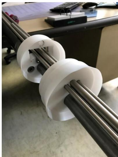
Figure 15: Hydrating system composed of (i) PTFE skirt-shape sealing system (white parts) and (ii) three stainless-steel lines.
