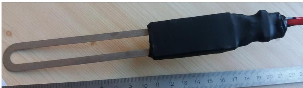
Figure 14: Electrical Resistance (ER) corrosion sensors (developed by ZAG)
