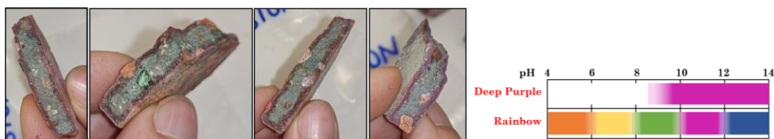
Figure 3-11 pH determination of LPC_SURAO by rainbow indicator (T3 – 18 months aged samples; broken discs after punch tests).
