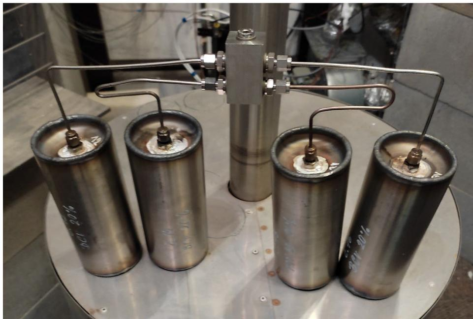
Figure 5-3. Steel vessels containing steel cells connected by metal capillaries with saturation medium situated in the irradiation area.
