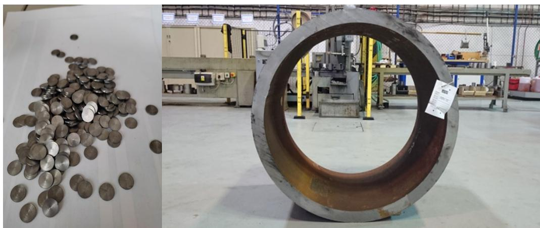
Figure 5-1. Left – carbon steel disks, right – outer case of the canister in the Czech concept.
