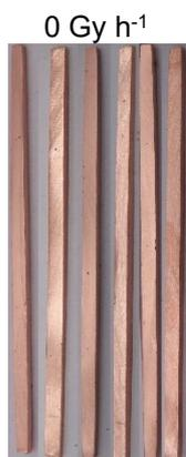
Figure 3-11. Wrought copper samples exposed for 1 h at 0 Gy h<sup>-1</sup> (WC1-1). Note replica samples #1 - #6, as denoted in Section 2.4, are positioned from left to right.
