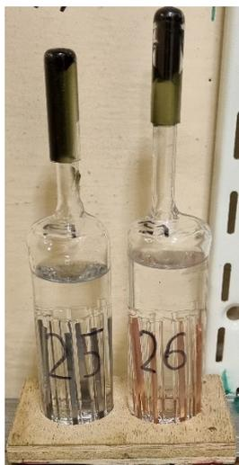
Figure 2-3. Ampoules 25 and 26 (Design One) with carbon steel and wrought copper specimens/cold-sprayed copper specimens immersed in the buffer solution.
