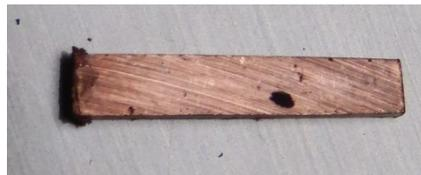
Figure 3-25. An optical image of a sample sub-section from a wrought copper sample exposed to a dose rate of 0.2 Gy h<sup>-1</sup> for 5000 hours (WC5-3#1C) analysed with SEM/EDX and Raman spectroscopy.
