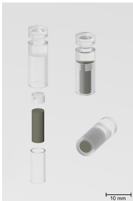
Figure 1: Schematic illustration of the preparation of in-diffusion samples in a filter-free approach. Left (from top): sample holder (PMMA, OD 8.0 mm, ID 6.0 mm, L 24.0 mm); optional centering sleeve, covering the upper part of the OPA cylinder ( \varnothing 5.0 mm, L (max.) 13.0 mm); structure below visualizing the interspace between OPA and sample holder, filled with epoxy resin. Upper right: compound sample with embedded OPA cylinder and optional centering sleeve. Lower right: rotated compound sample with exposed OPA in-diffusion surface. Visualization generated with Blender (2023).
