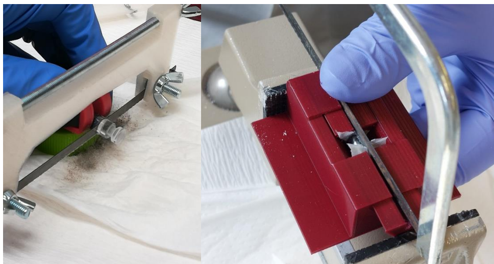
Figure 4: Preparation of an in-diffusion sample for TOF-SIMS measurements. After an initial decontamination of the outer sample holder, the sample is immediately processed, preferably preserving the saturated state of the embedded OPA clay rock. Left: Detaching the upper mounting part (PMMA) of the sample. Right: Isolated subsample mounted in a 3D printed cleaving tool. Sawing of the outer PMMA and resin layer parallel to the bedding. The picture is showing an earlier test without deployed activity. Subsequent processing of in-diffusion samples with ^{239}\text{Pu} was done in the controlled environment of a fume hood, considering the generation of sawdust.
