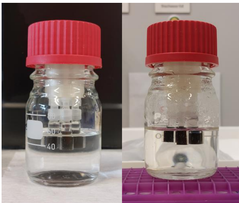
Figure 2: In-diffusion setup (left) during the resaturation/conditioning phase and (right) during the in-diffusion experiment. Standard borosilicate glass laboratory bottle (100 mL), 3D printed insert and mounted samples, immersed in OPA pore water respectively a diffusion solution of ^{239}\text{Pu(IV)} in OPA pore water. Minor condensation at the inner glass wall of the bottle could be observed due to the thermal discharge of the magnetic stirrer. The bottle is placed on a grid allowing a better ventilation of the experiment.
