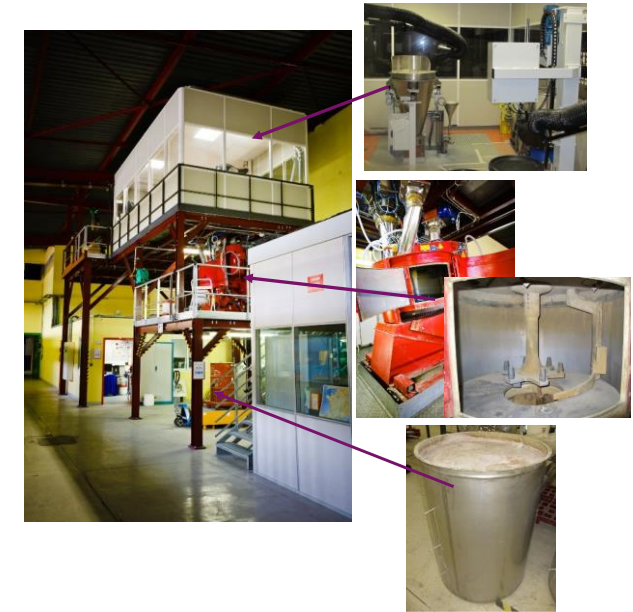
In-line mixing using a high shear mixer – STEMA platform
