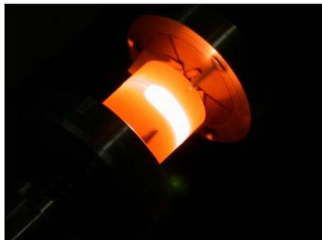
Joining process of SiC-capsule
