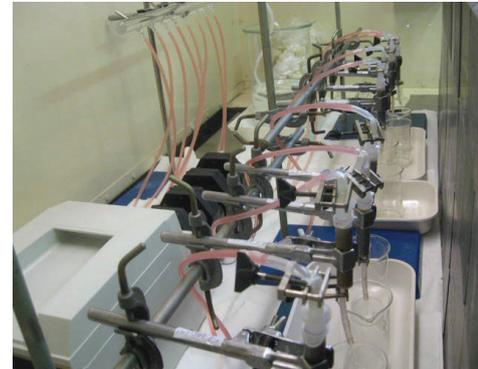
Fig. 2. Instrumental set-up of column experiments
