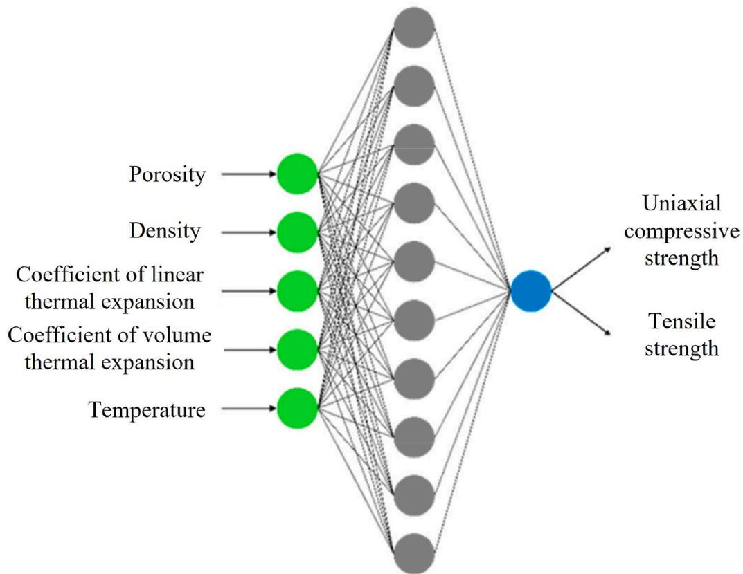
Fig. 6. Artificial neural network (ANN): using five input parameters to predict strength properties of thermally treated sandstone (Sirdesai et al., 2019).
