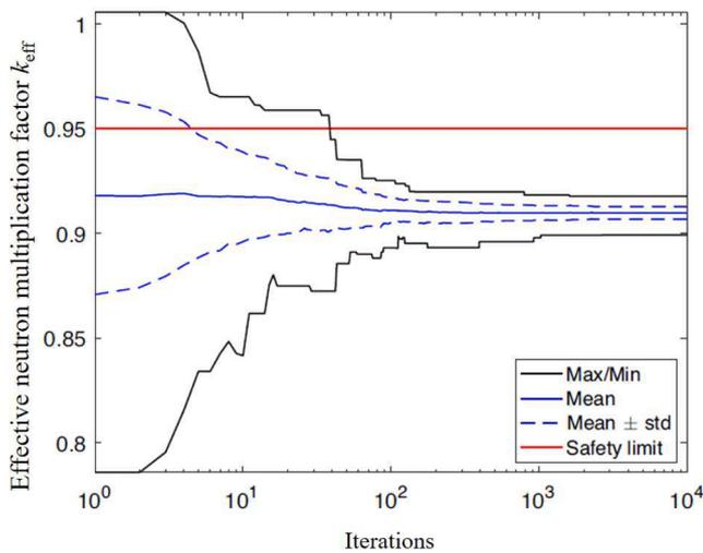
Fig. 7. Genetic algorithm (GA): mean value and standard deviation of  $k_{eff}$  change with iterations (Solans et al., 2021).
