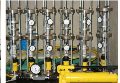
Experimental setup for the triaxial (left) and creep tests (right) Ecole centrale des Mines
