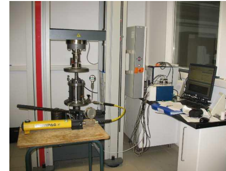
Experimental setup for the triaxial (left) and creep tests (right) Ecole centrale des Mines
