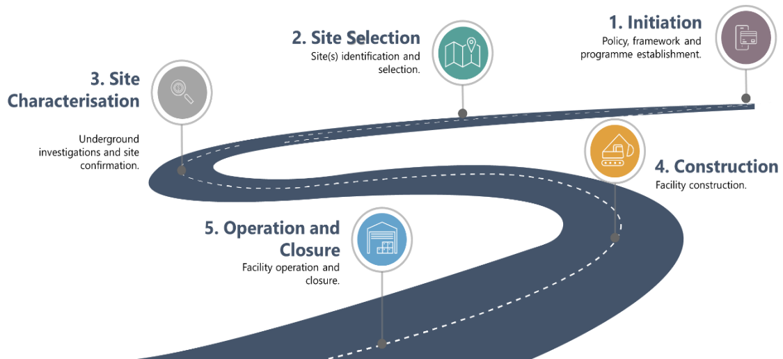
Figure 1: Phases of implementing a deep geological repository programme, adapted from the IAEA DGR Roadmap (IAEA, 2021). Note: Phases are not necessarily discrete but often overlap and are typically iterative (i.e., not simply sequential), and can differ from country to country.
