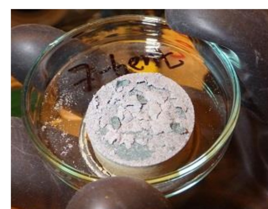
Fig. 4 Compacted bentonite with a layer of a mixture of Fe powder and corrosion products; lab temperature, 189 days; CoPr experiment.
