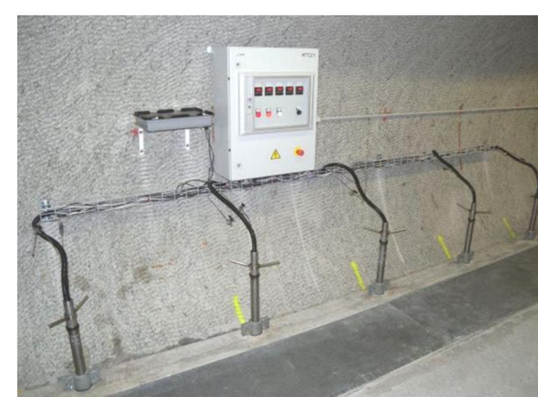
Fig. 2 Emplacement of samples in five boreholes at GTS (MaCoTe)
