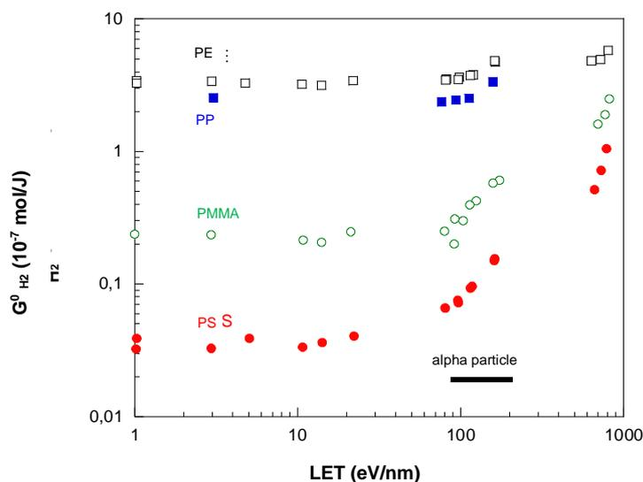
FIGURE 2-5. Variation of H<sub>2</sub> production yields as function of LET for polyethylene (PE), polypropylene (PP), poly(methyl methacrylate) (PMMA) and polystyrene (PS) (Chang & Laverne, 2000).
