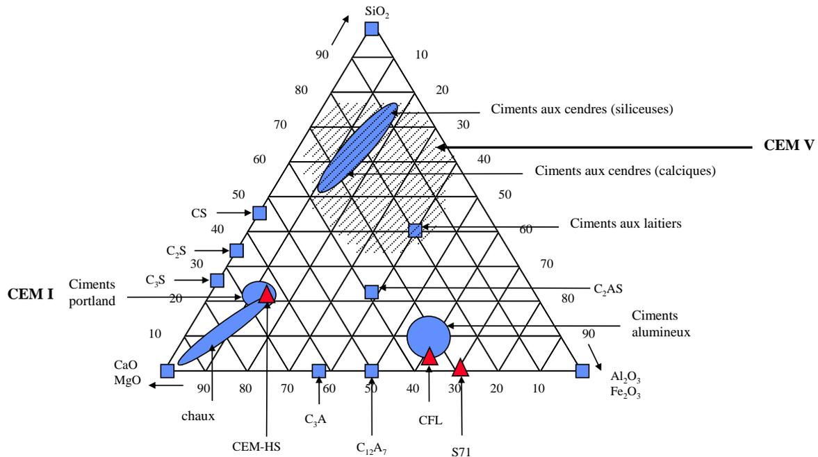
FIGURE 5-1: Ternary diagram CaO-SiO<sub>2</sub>-Al<sub>2</sub>O<sub>3</sub> showing the compositions of the main types of cement (from Damtoft *et al.*, 1999).
