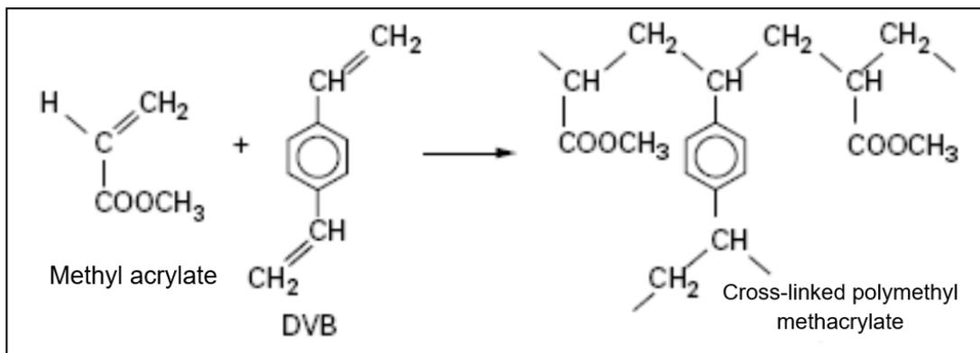
**FIGURE 2-4:** Formation of a polyacrylic skeleton (De Dardel, 1998).
